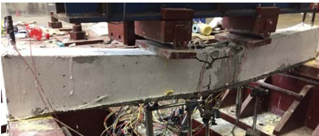
Fig. 5. Failure mode of tested beams
