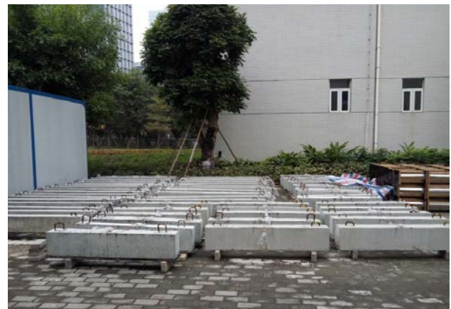
Fig. 2. Specimens under accelerated corrosion process in the open air space
