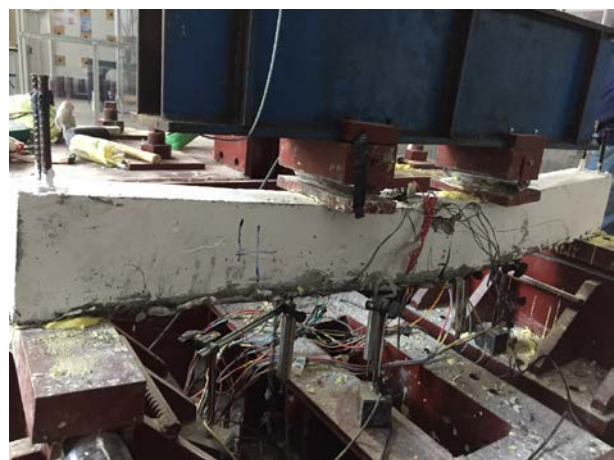
Fig. 4. Four-point bending test set-up
