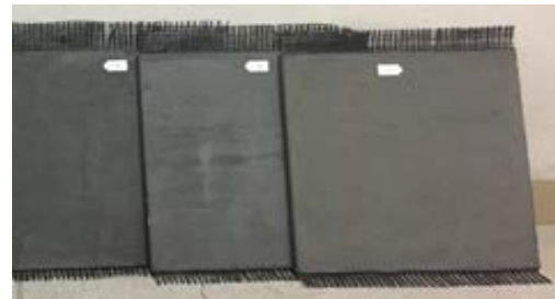
Fig. 1. Carbon-fiber reinforced cementitious matrix (C-FRCM) manufactured in the laboratory
