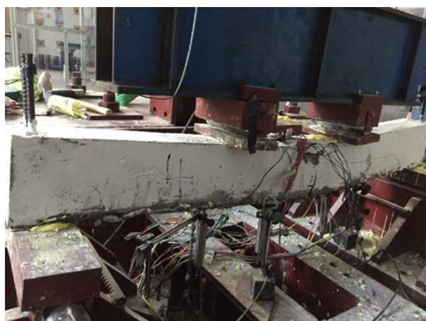
**Fig. 4.** Four-point bending test set-up
