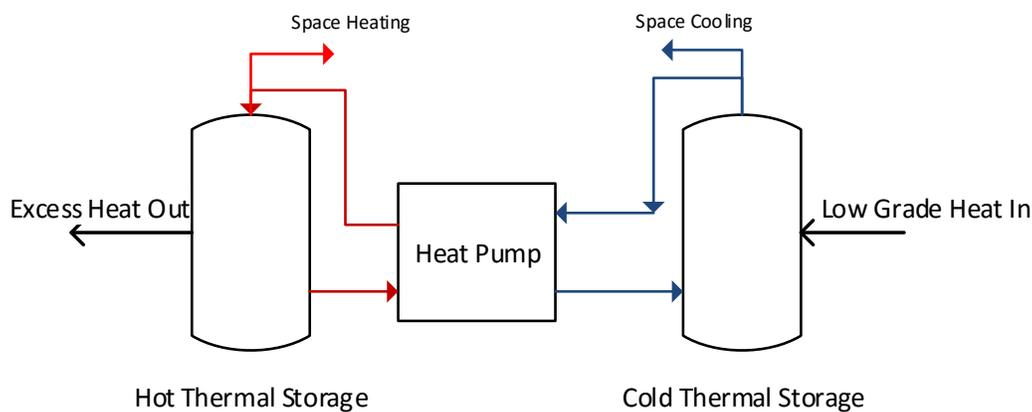
**Figure 1:** High level schematic of proposed system
