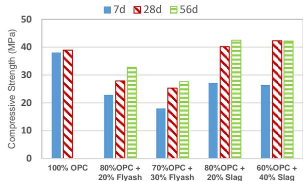
Fig. 3. Comparison of strength development in concrete with different replacement levels of Fly ash and slag
