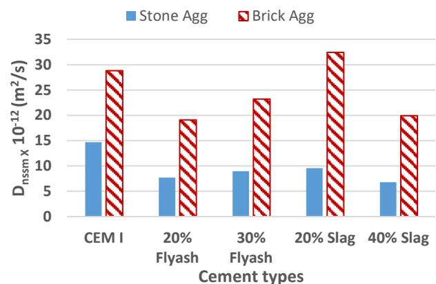
**Fig. 4.** Comparison of Migration coefficient for different concrete mixes with 350 kg/m<sup>3</sup> cement content
