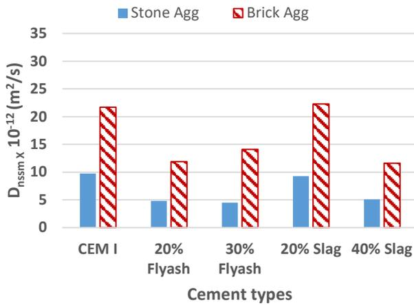
**Fig. 5.** Comparison of Migration coefficient for different concrete mixes with 450 kg/m<sup>3</sup> cement content
