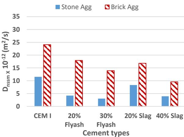
**Fig. 6.** Comparison of Migration coefficient for different concrete mixes with 550 kg/m<sup>3</sup> cement content
