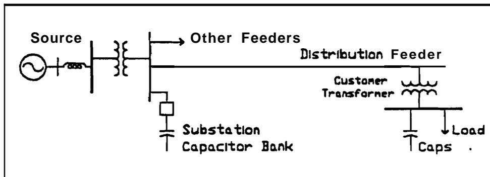
*Figure III.1 Single line diagram for example power system.*
