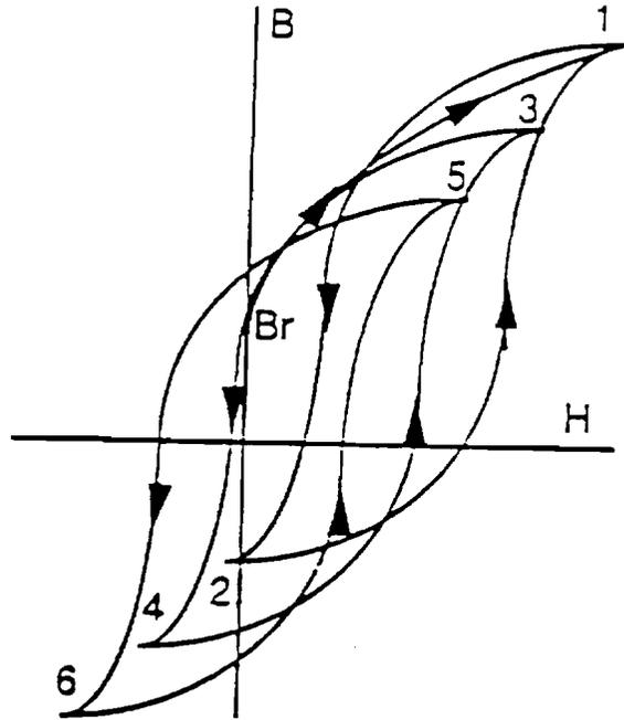
Figure V.1 The Magnetizing Characteristics of a Transformer.
