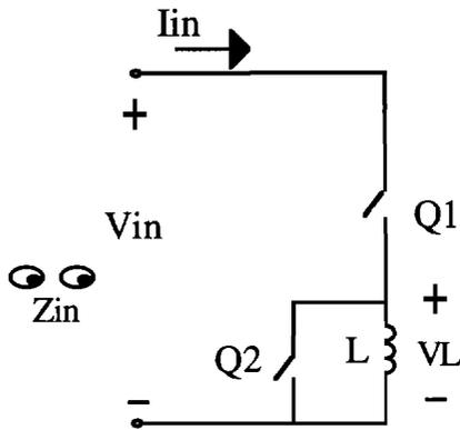
If the effect of high-order switching harmonics is neglected, the inductor voltage and input current can be expressed as:
