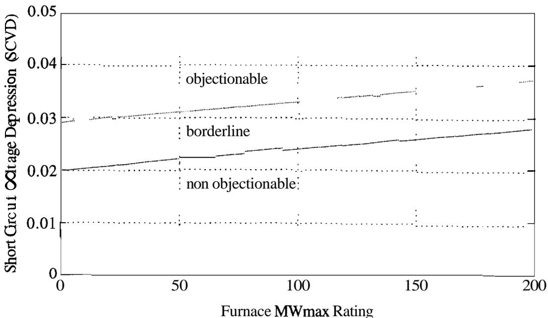
Fig. IV.3 SCVD as a function of furnace MWmax
