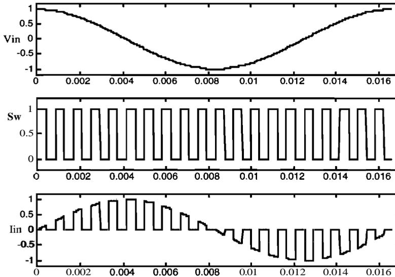
The last equation shows that the input equivalent reactance can be expressed as a function of the inductor reactance and the switching duty cycle. In other words, the reactive power of this circuit can be adjusted through duty cycle control. [6]
