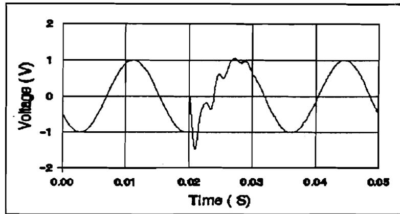
Figure III.5 Transient voltage at the switched shunt capacitor.
