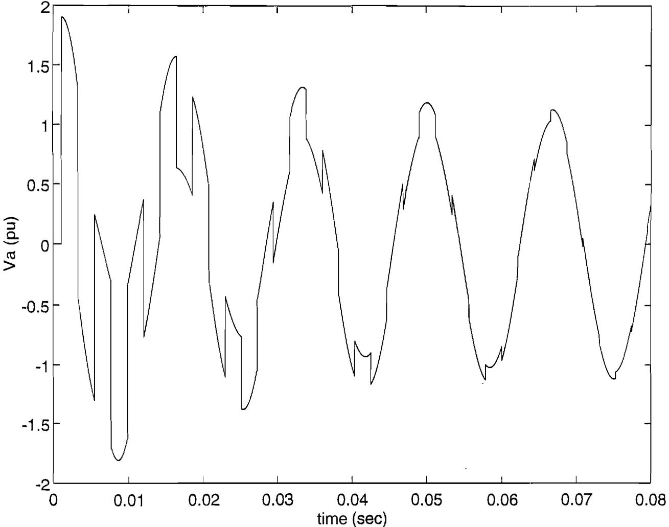
Figure VI.4  $V_a$  receiving end for simultaneous pole closure:
