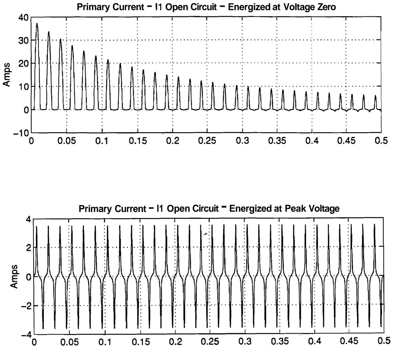
Figure V.4 Simulation Results of the Open Circuit Condition.
