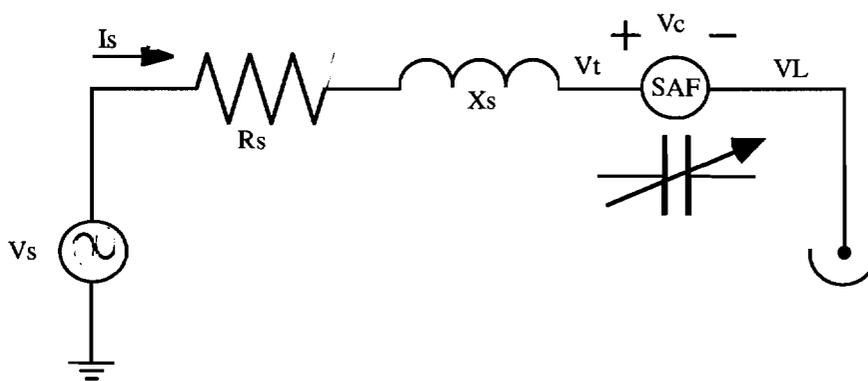
Fig. IV.6 Single phase equivalent circuit of proposed system.
