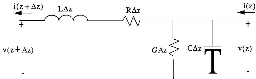
Figure VI.1 Single-phase transmission line differential section equivalent circuit
