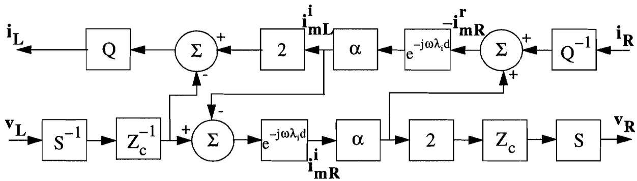
Figure VI.2 Block Diagram for Transmission Line Simulation
