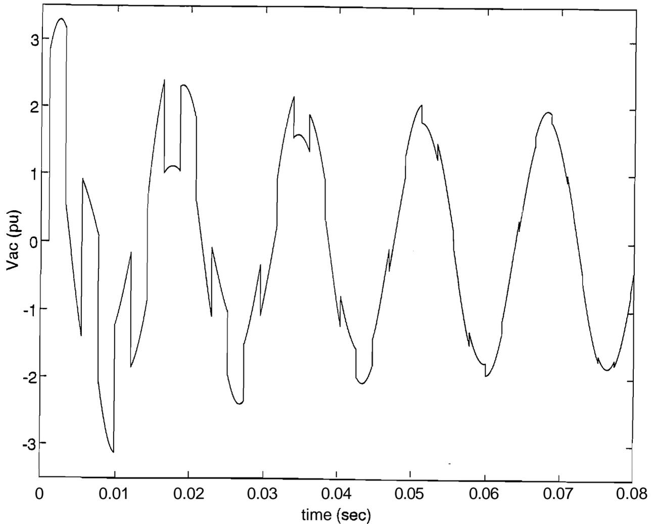
Figure VI.5  $V_{ac}$  receiving end for simultaneous pole closure
