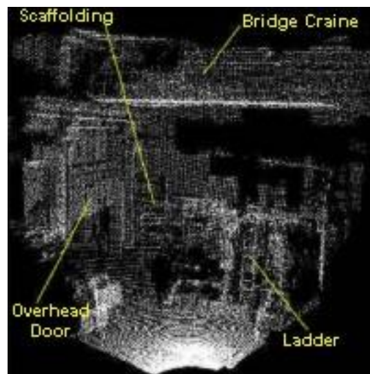
FIGURE 1 ACTUAL LIDAR SCAN: THIS IMAGE PROVIDES AN EXAMPLE OF THE DENSE CLUTTER TO BE EXPECTED AT AN EVERYDAY CONSTRUCTION SITE
