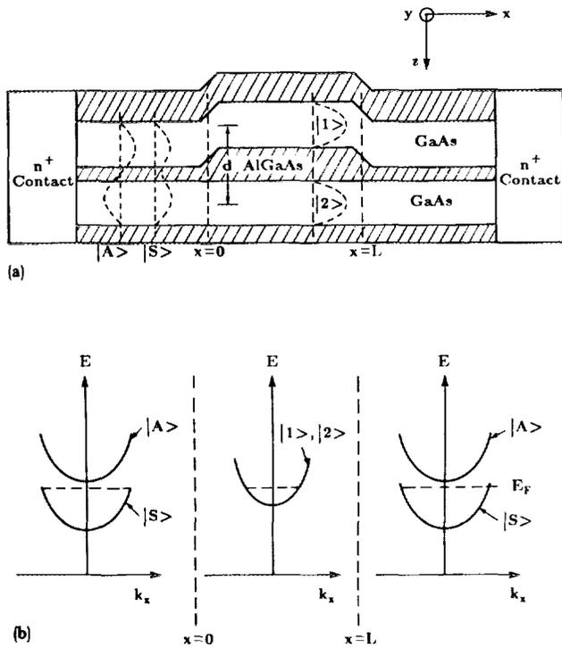
FIG. 1. Proposed structure. (a) Configuration: The current flow is in the  $x$ - $y$  plane along the two GaAs quantum wells.  $|S\rangle$  and  $|A\rangle$  represent the wave functions in the  $z$  direction for the two lowest transverse modes in the end regions. In the central regions the eigenmodes  $|1\rangle$  and  $|2\rangle$  are isolated and degenerate. (b)  $E$  vs  $k_x$  at different points for the different transverse eigenmodes.
