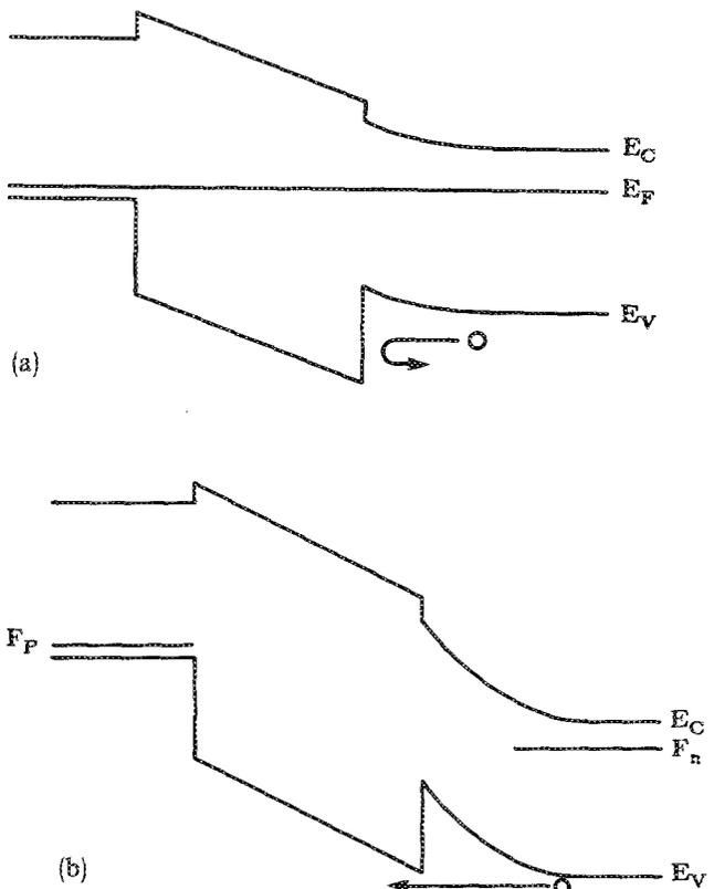
FIG. 5. Energy-band diagrams of the  $p^+in$  GaAs/AlAs/GaAs photodiode: (a) zero-bias condition; (b) biased to where the valence-band discontinuity is equal to the band bending in the  $n$  GaAs buffer region.
