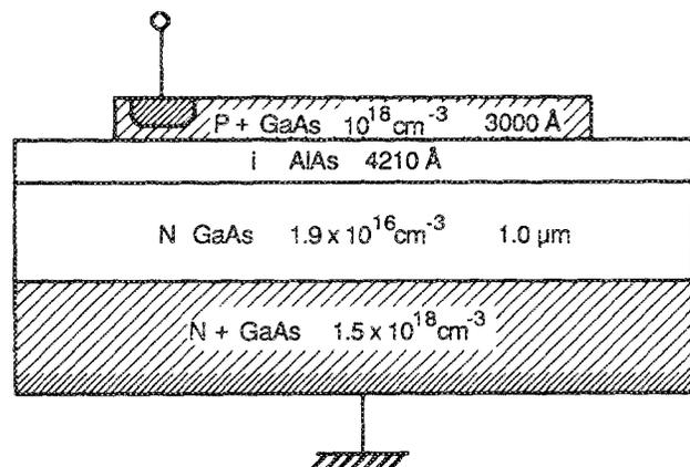
FIG. 1.  $p^+$  in GaAs/AlAs/GaAs device structure.
