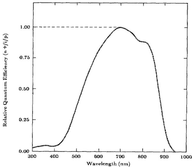
FIG. 3. Relative photocollection efficiency for an  $n^+ip$  GaAs/AlAs/GaAs photodiode. The top  $n^+$  GaAs layer was 3000 Å thick and the AlAs layer was 2800 Å thick.
