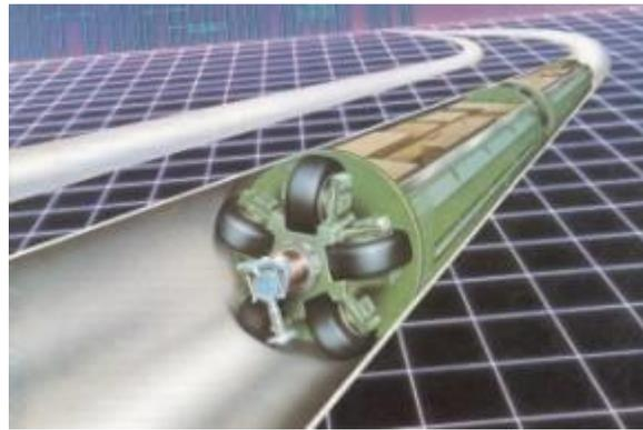
FIGURE 1 PCP WHEELED CAPSULE (DRAWING BY SUMITOMO METALS)
