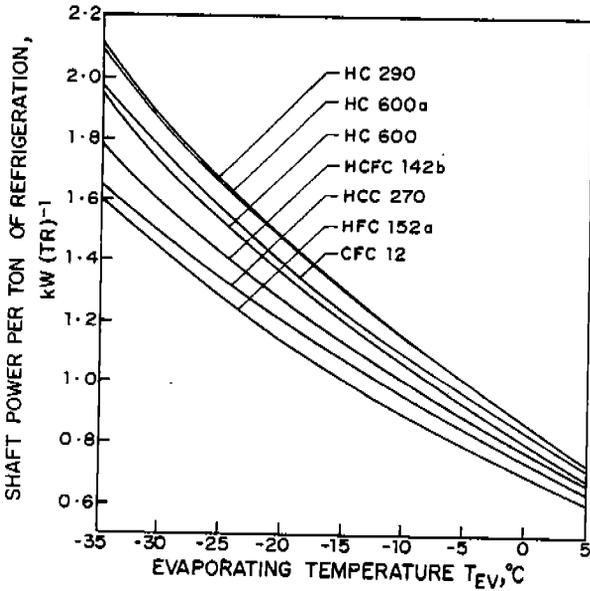
FIG. 4: W AGAINST  $T_{EV}$  FOR  $T_{CO} = 50^{\circ}C$
