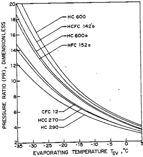
FIG. 1: (PR) AGAINST  $T_{EV}$  FOR  $T_{CO} = 50^{\circ}\text{C}$
