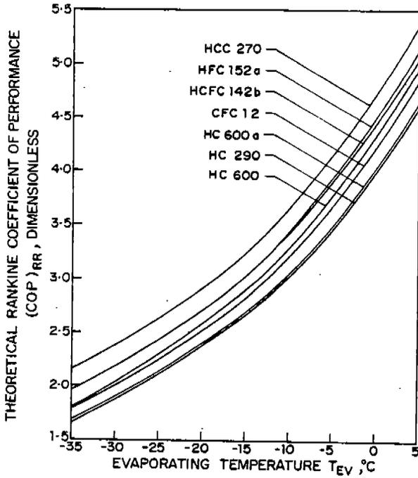
FIG. 3:  $(COP)_{RR}$  AGAINST  $T_{EV}$  FOR  $T_{CO} = 50^{\circ}C$
