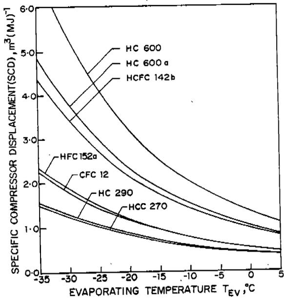
FIG. 2: (SCD) AGAINST  $T_{EV}$  FOR  $T_{CO} = 50^{\circ}\text{C}$
