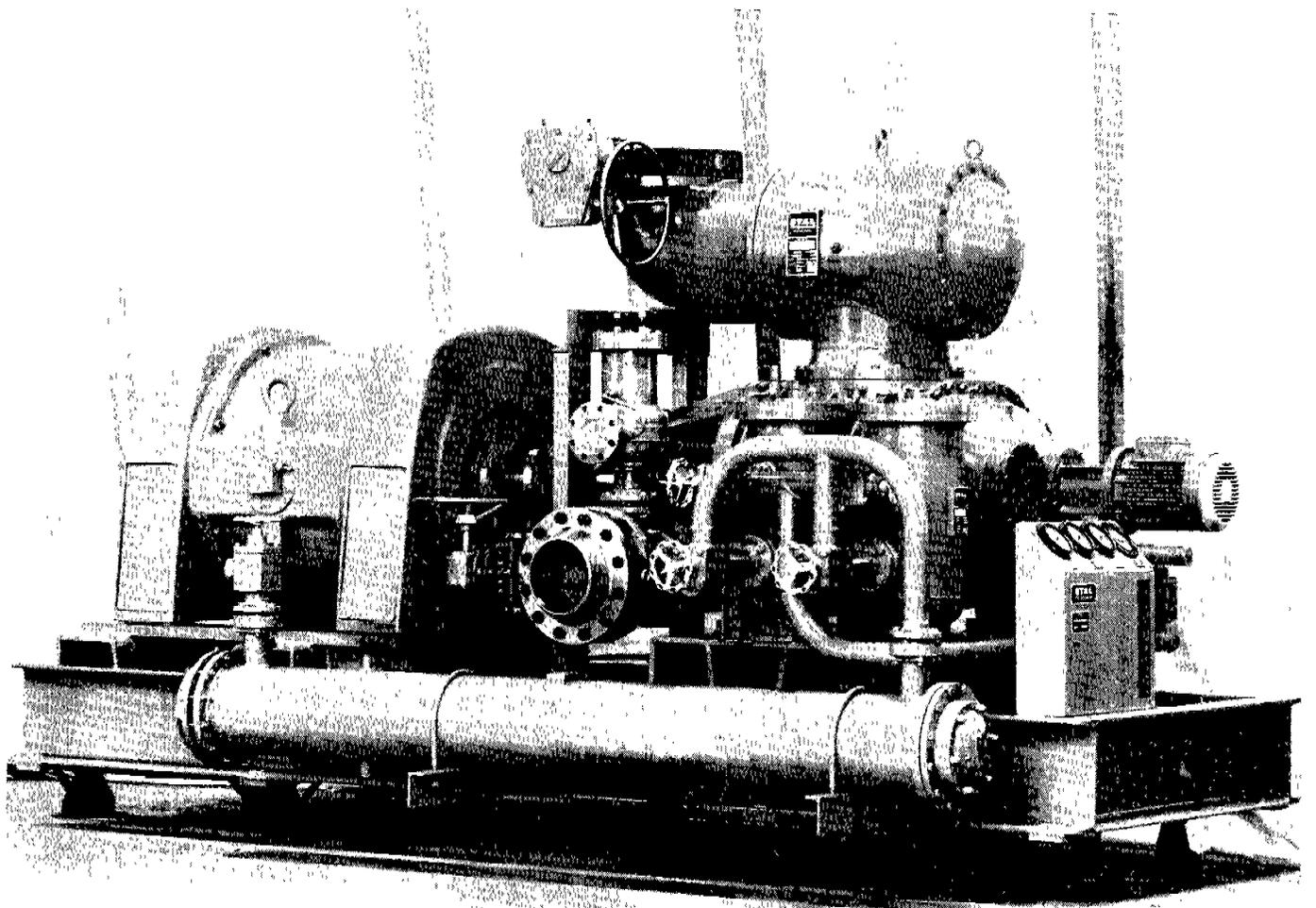
Figure 3 STAL Screw Compressor Type S93 Having 6900 m<sup>3</sup>/h Displacement
