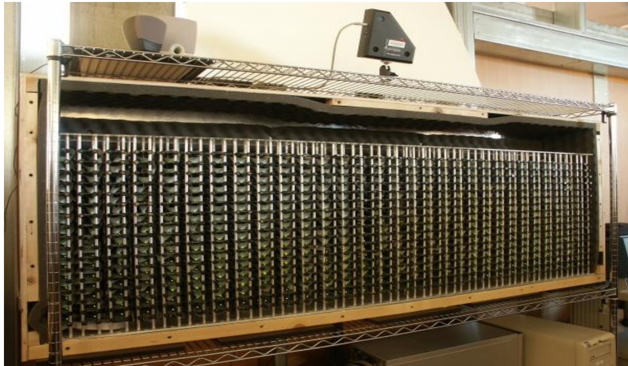
LOUD 1020-node microphone array
