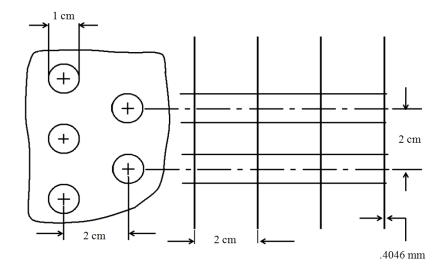
Figure 5. Heat exchanger geometry in a modified solar tower.
