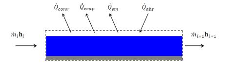
Figure 1. Control volume for one canal segment.
