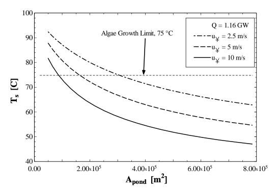
Figure 9. Algae bioreactor pond temperature versus pond area for various wind speeds.
