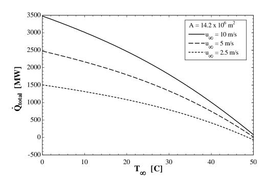
Figure 8. Total canal heat transfer versus ambient temperature for various wind speeds.
