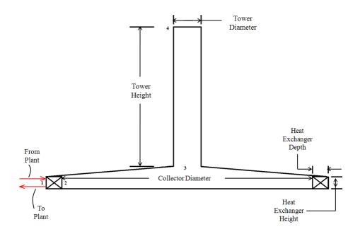
Figure 4. Modified solar tower schematic figure.
