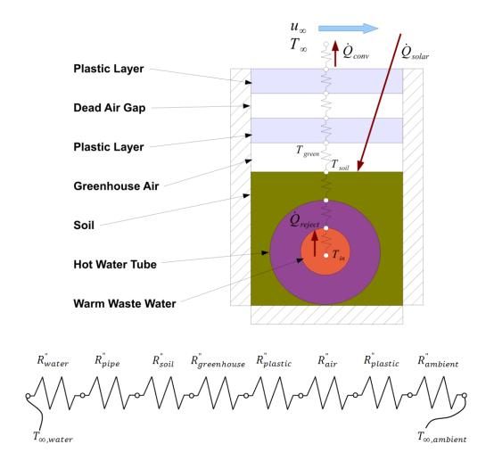
Figure 3. Greenhouse thermal resistance network.
