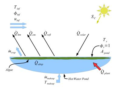
Figure 2. Algae bioreactor pond control volume.
