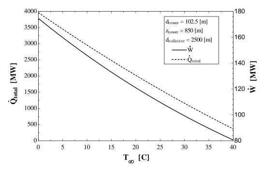
Figure 11. Modified solar tower heat rejection and power production versus ambient temperature.
