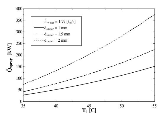
Figure 10. Spray heat transfer for a single nozzle versus condenser discharge temperature for various droplet diameters.
