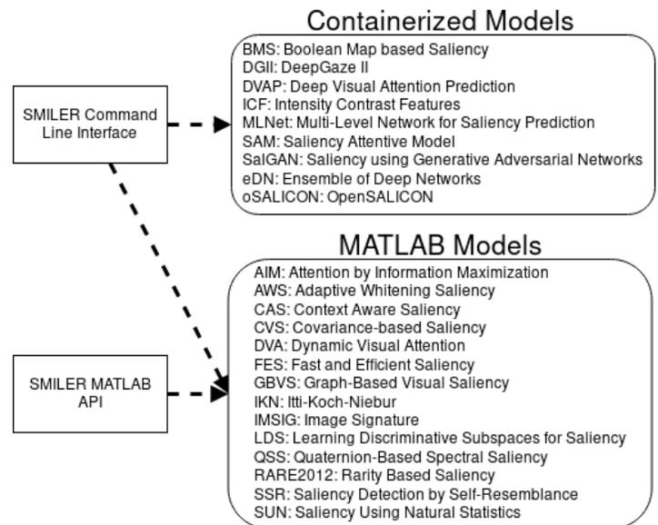
Figure 1: Diagram showing model implementations and interfaces provided by the SMILER system.
