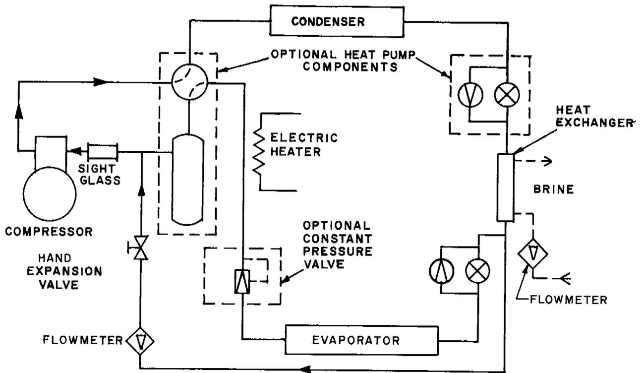
Figure 6. Refrigerant Piping Schematic
