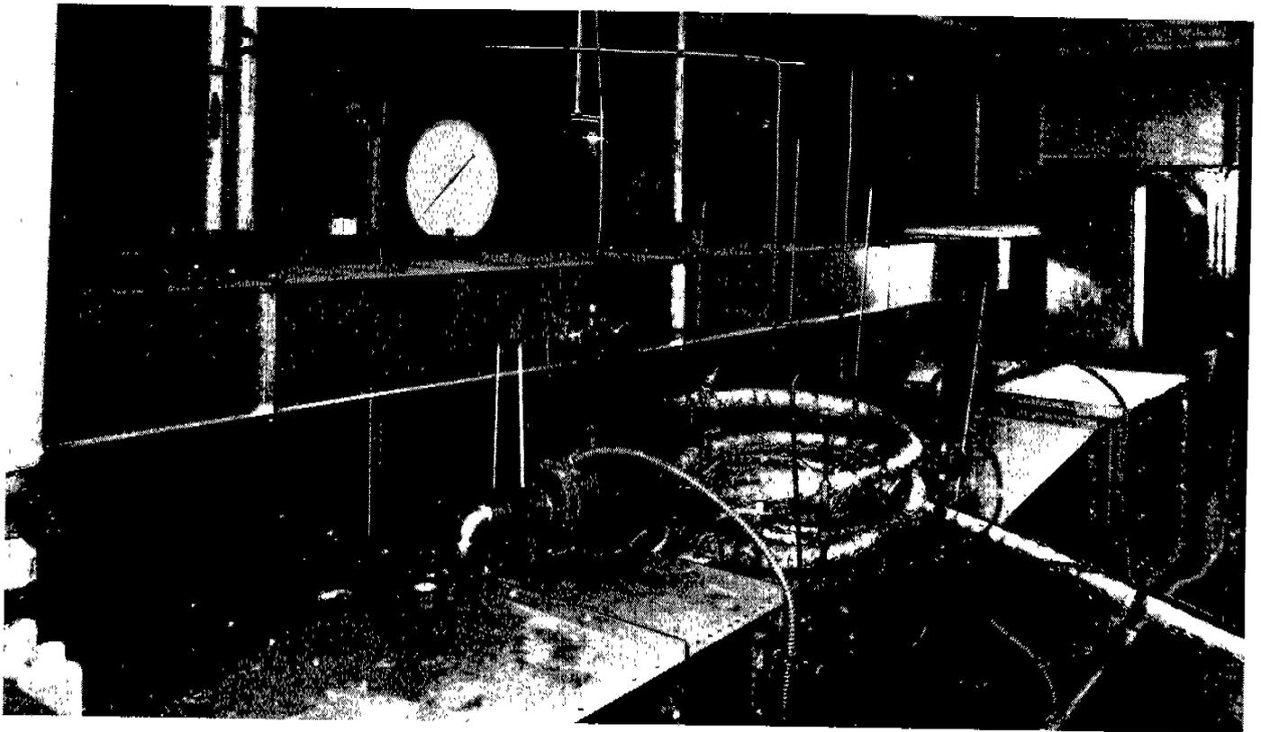
Figure 7. Evaporator Test Loop, Showing Coiled Liquid and Suction Line Heat Exchangers
