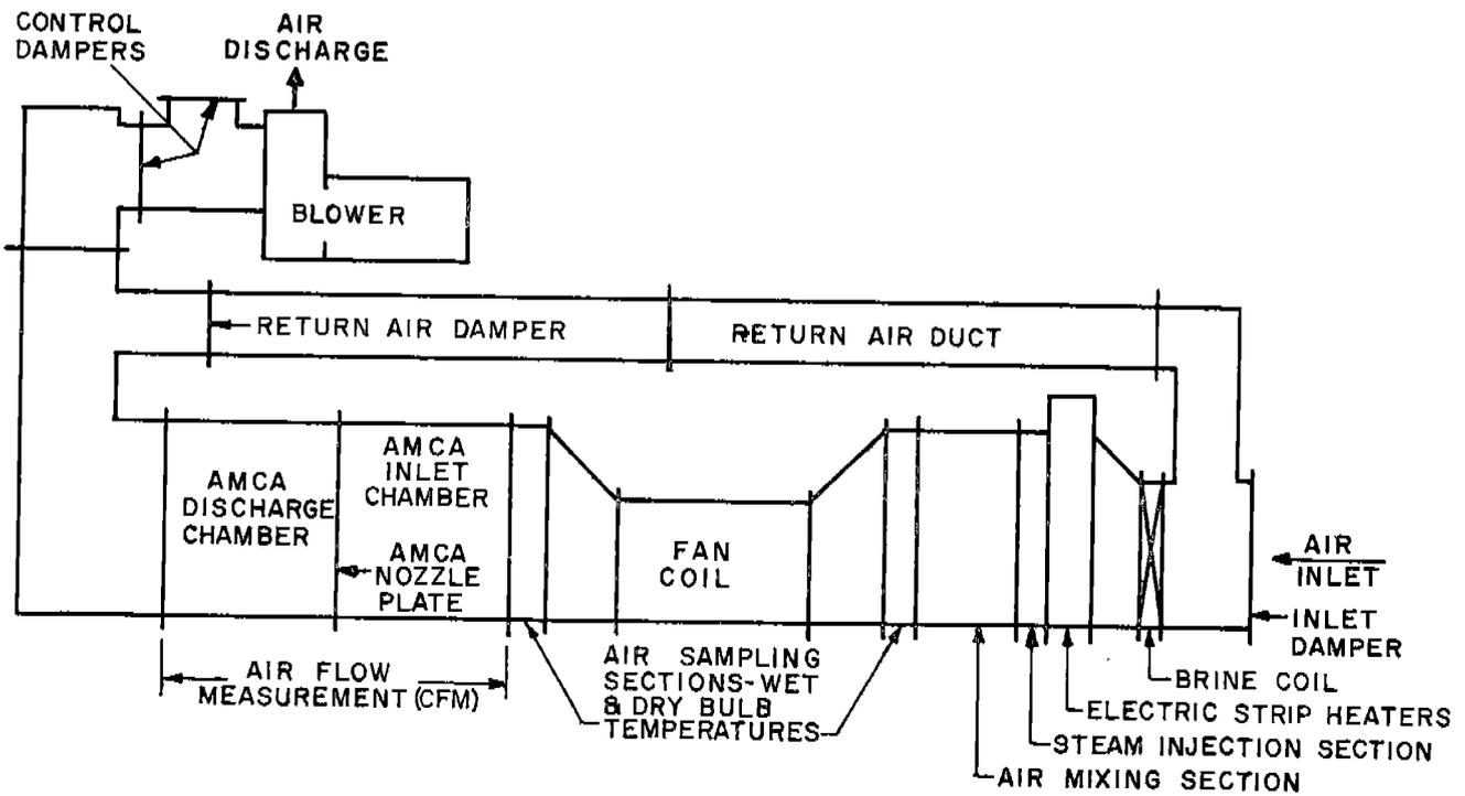
Figure 4. Evaporator Test Loop
