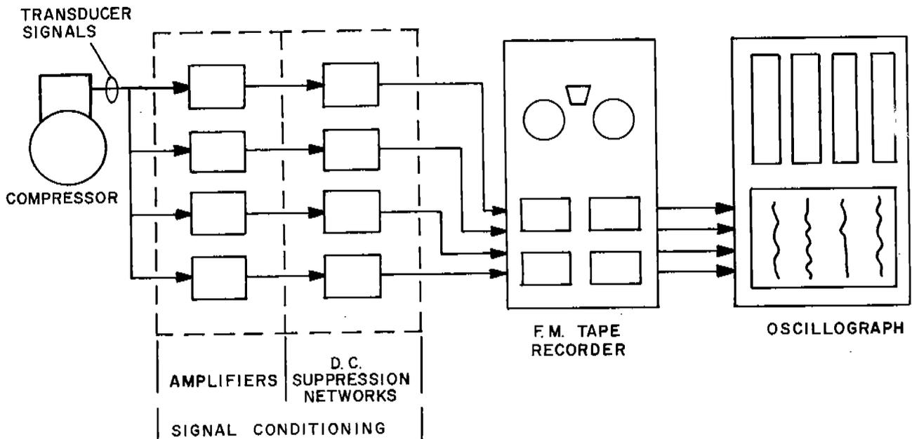
Figure 9. Instrumentation Schematic
