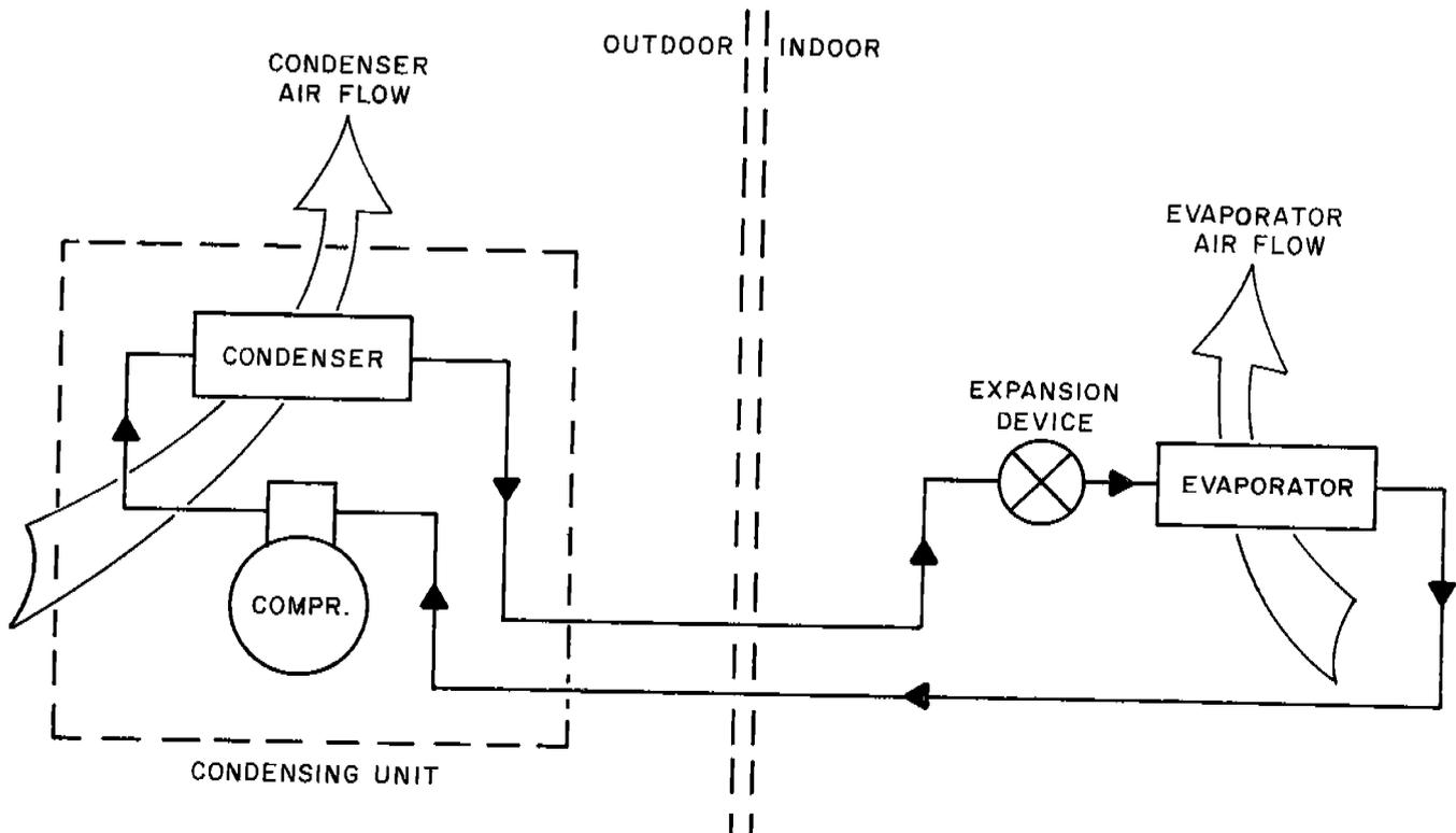
Figure 1. Typical Components and Arrangement for Residential Split-System Air Conditioners
