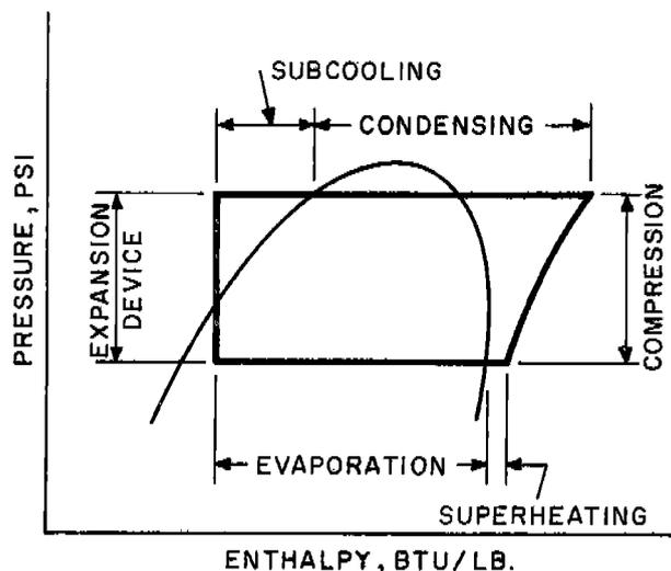
Figure 2. Pressure-Enthalpy Diagram for Air Conditioning Vapor Compression Cycle
