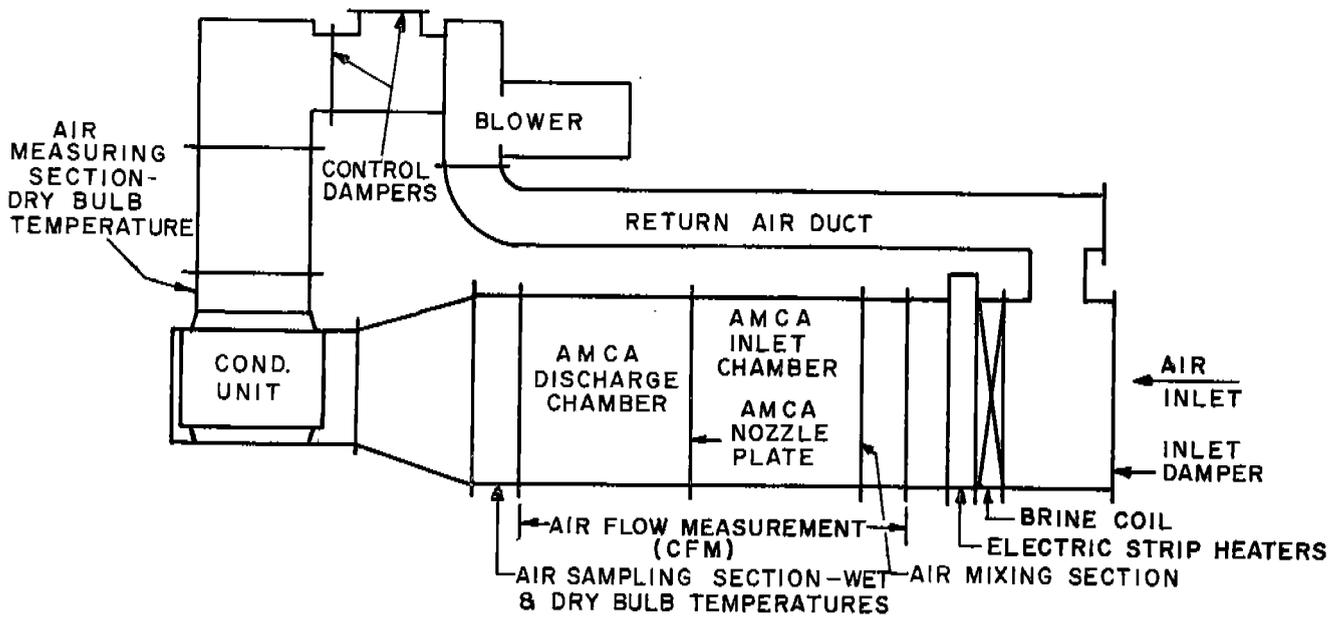
Figure 3. Condenser Test Loop
