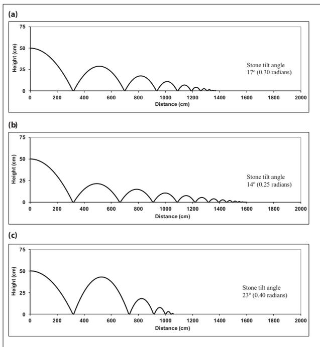
**Fig. 5.** Typical stone trajectories for the standard model. Note the difference in horizontal and vertical length scales, which exaggerates apparent skip height. Minimum legal skip height,  $y_{\text{legal}} = 0$ . Other model parameters are those listed in Table I. (a) Tilt angle =  $17^\circ$  (0.3 rad). (b) Tilt angle  $\alpha = 14^\circ$  (0.25 rad). (c) Tilt angle  $\alpha = 23^\circ$  (0.4 rad).
