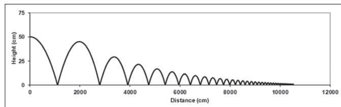
Fig. 1. Trajectory of a skipping stone with parameters of a championship throw. Launch speed 3600 cm/s. Note difference in horizontal and vertical distance scales, which distorts the apparent heights of the skips.
