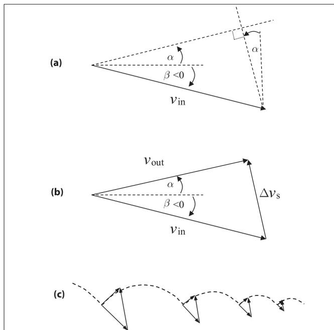
**Fig. 4. (a) and (b) Vector addition  $v_{in} + \Delta v_s = v_{out}$  for computing outbound velocity of a skipping stone. (c) Serial application of the vector addition rule to reconstruct airborne segments of the stone's trajectory.**
