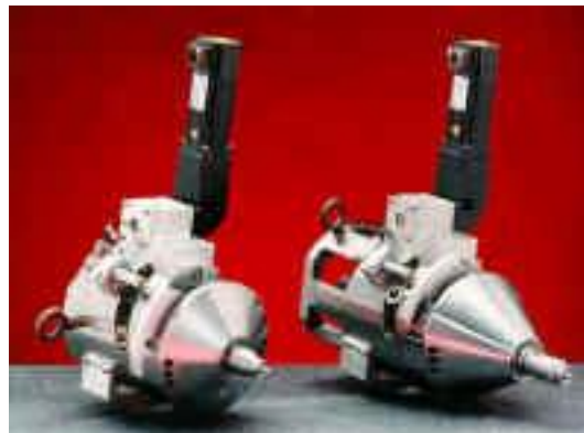
FIGURE 2 RETRACTABLE PIN TOOL (COURTESY OF NASA MARSHALL SPACE FLIGHT CENTER)
