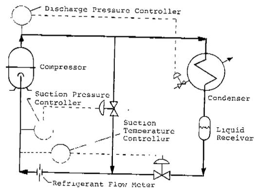
Figure 1. Schematic of Gaseous Refrigerant Flow Meter Calorimeter
