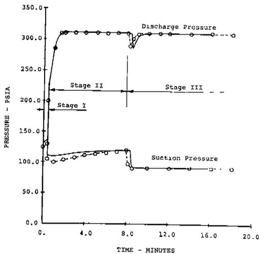
Figure 7. Compressor Discharge and Suction Pressures vs Time
