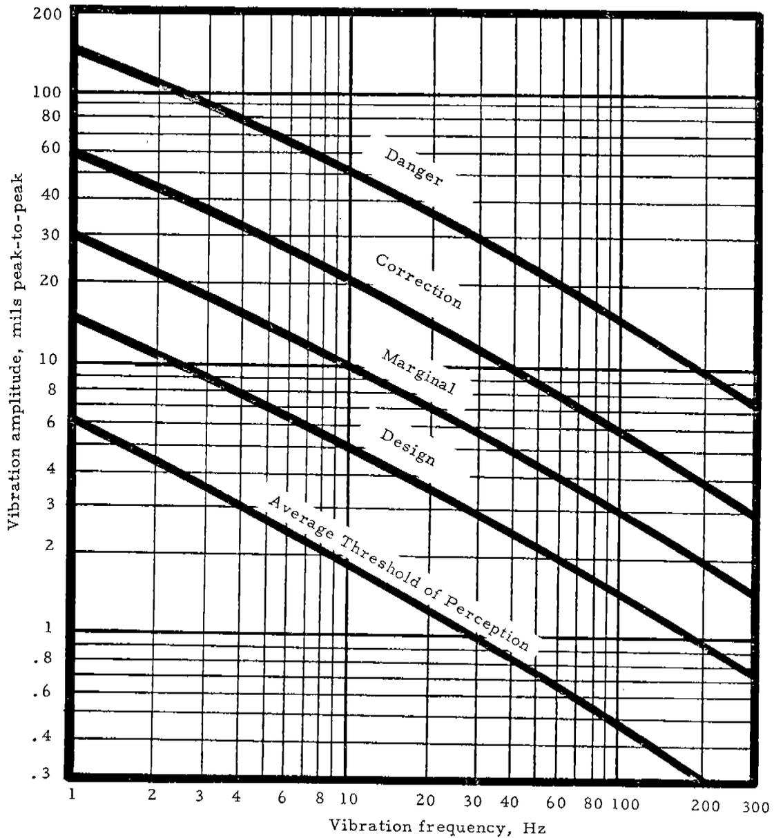
Note: Indicated vibration limits are for average piping system constructed in accordance with good engineering practices. Make additional allowances for critical applications, unreinforced branch connections, etc.
