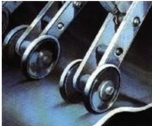
FIGURE 2 CALSCAN: DETECTING DENTS - PIPETRONIX INC
