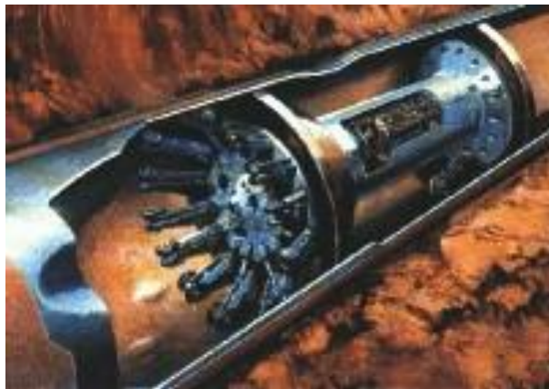
FIGURE 1 CALSCAN SMART PIG - PIPETRONIX INC
