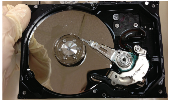
A hard drive damaged by silt and then shown again after being cleaned with a series of organic solvent rinses.
