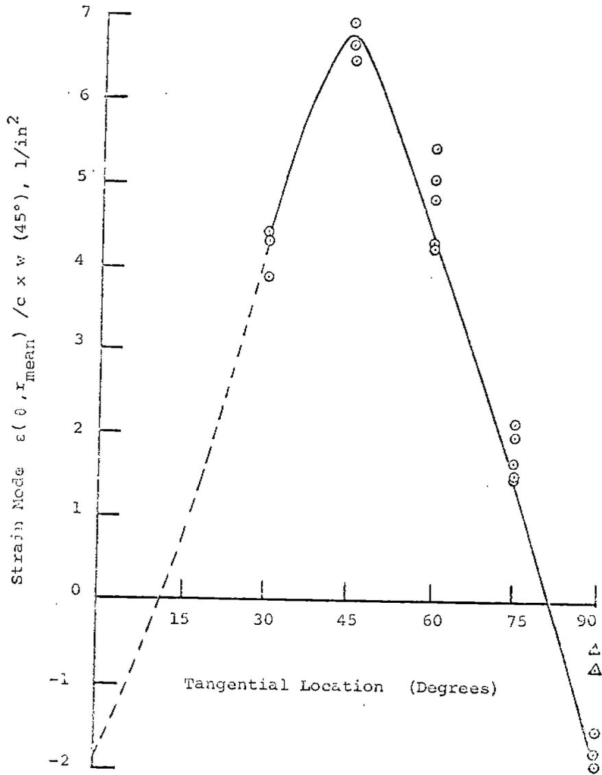
Figure 5. Measured Strain Mode  $\psi_{41}$  For Suction Valve in Four Point Support Boundary
