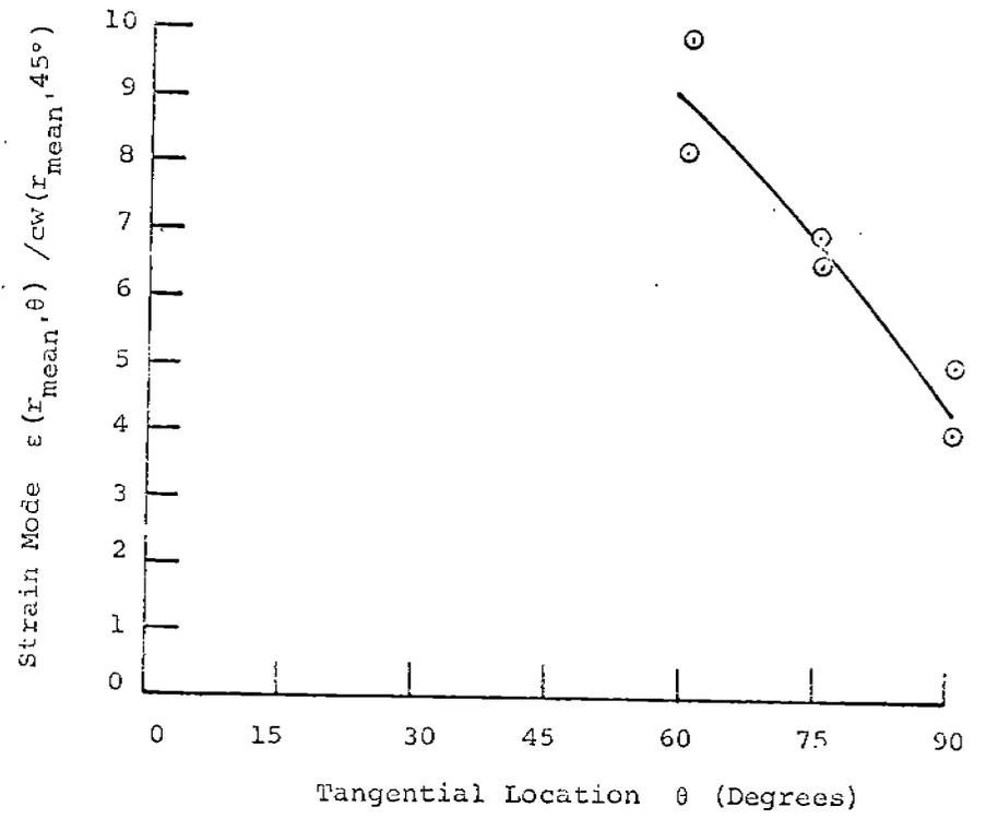
Figure 6. Measured Strain Mode  $\psi_{42}$  for Suction Valve in Four Point Support Boundary
