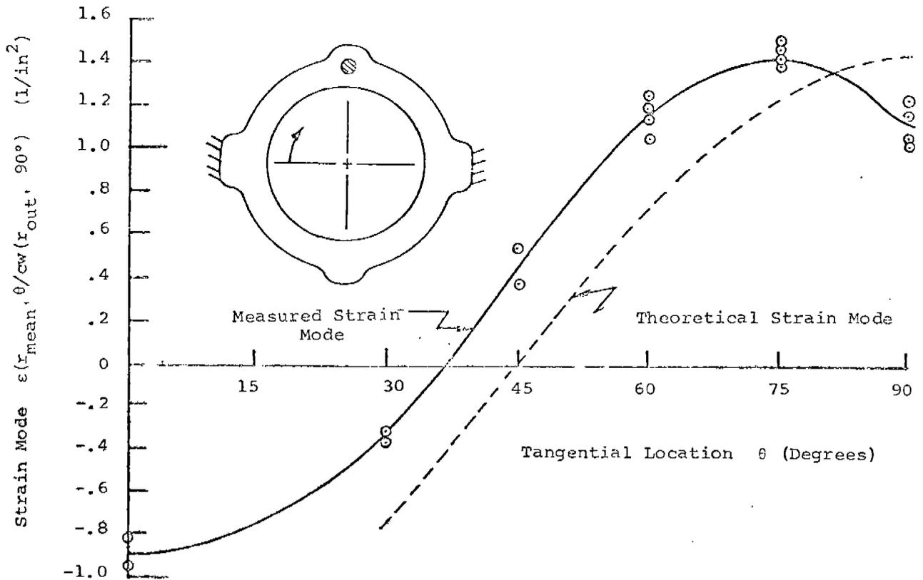
Figure 4. Measured Strain Mode  $\phi_{21}$  For Suction Valve in Two Point Support Boundary
