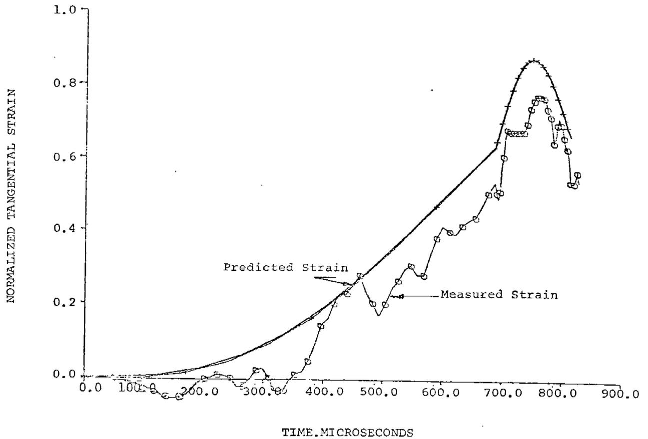
Figure 8. Total Strain Prediction Using First Two Symmetric Overshoot Modes
