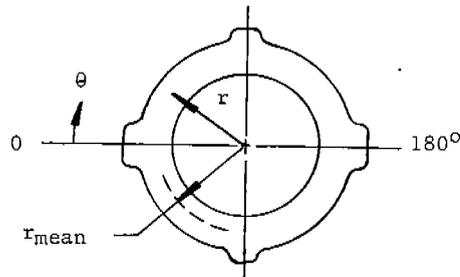
Figure 1 Ring Valve in Polar Coordinates
