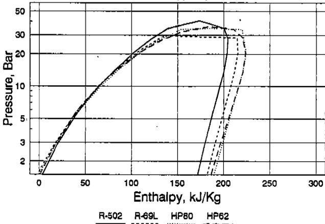
Figure C. Pressure-Enthalpy Diagram for R-502 and R-502 Alternatives.
