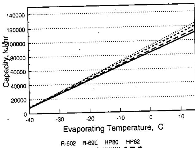
Figure D. Theoretical Capacity of R-502 and R-502 Alternatives at Various Evaporating Temperature. Condensing Temperature is 43.3 C. Compressor Displacement is 25 cubic meters per hour.
