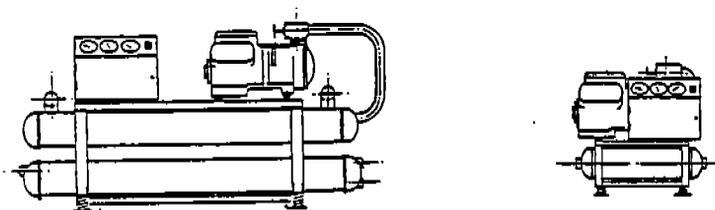
FIG 6 EFFECT OF PCHE ON PLANT SIZE (from Johnston (1985))
