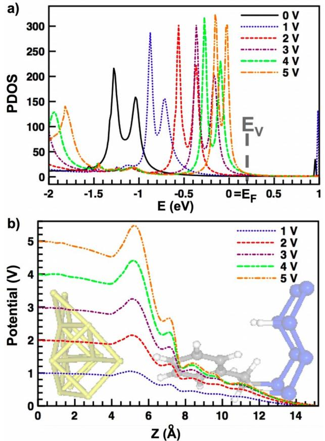
FIG. 6. (Color online) Bias characteristics of styrene attached to Si(100) in physisorption contact (full contact) with a Pt(100) tip. The PDOS of the styrene  $\pi$  state under bias is shown in (a). The potential profile across the device region is shown in (b), where a cut of the potential drop is taken through the tip apex atom. The electrochemical potential is located at  $-5.2$  eV.
