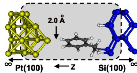
FIG. 2. (Color online) Simulated two-probe transport structure for styrene on Si(100) beneath a Pt(100) tip. The tip position of closest approach is set at 2.0 Å above the highest styrene hydrogen atom.
