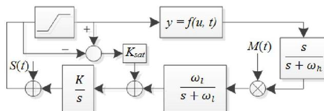
**Figure 4:** Anti-windup ESC
