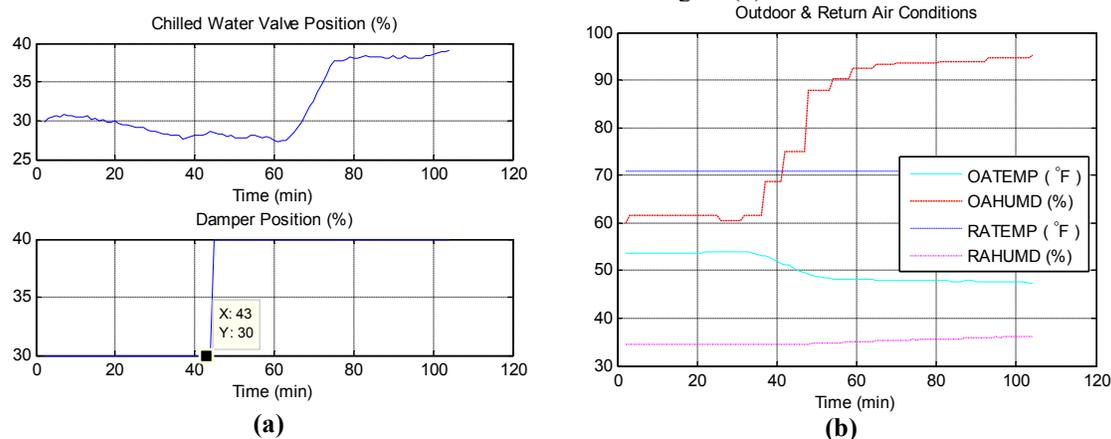
**Figure 10:** (a) Step test from damper opening to Chilled water valve position (b) outdoor air conditions and return air conditions
