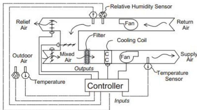
**Figure 1:** Single-duct of air-handling unit
