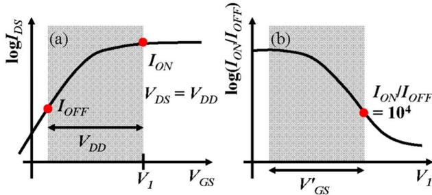
FIG. 1. Approach to compare the performance of 1D and 2D transistors. (a) For a given  $V_{DD}$ , the  $V_{DD}$  window is swept in  $I_{DS}$  vs  $V_{GS}$ . The right end of the  $V_{DD}$  window is denoted as  $V_I$ . (b) For a desired  $I_{on}/I_{off}$ , we choose a new gate bias range,  $V'_{GS}$ . Then, 1D and 2D transistors are compared in the gate bias ranges that give us the same  $I_{on}/I_{off}$ .
