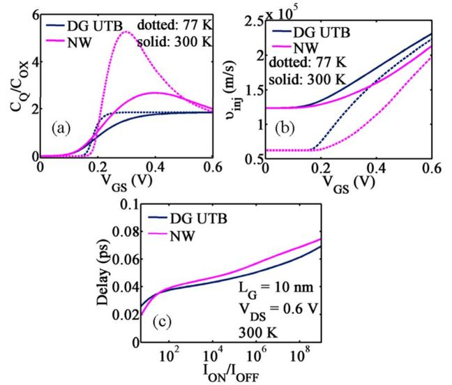
FIG. 3. Simulation results of (a)  $C_Q/C_{ox}$  vs  $V_{GS}$  at  $T = 77$  K and  $T = 300$  K, (b)  $v_{inj}$  vs  $V_{GS}$  at  $T = 77$  K and  $T = 300$  K, and (c) the intrinsic device delay vs  $I_{on}/I_{off}$  at  $T = 300$  K. Device dimension itself makes little difference to the device performance.
