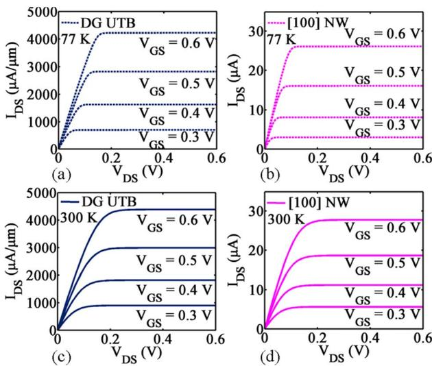
FIG. 2. Simulation results of  $I_{DS}$  vs  $V_{DS}$  of 1D and 2D silicon  $n$ -MOSFETs at  $T = 77$  K and  $T = 300$  K. In (c) and (d), the 1D and 2D transistor characteristics look similar at room temperature.
