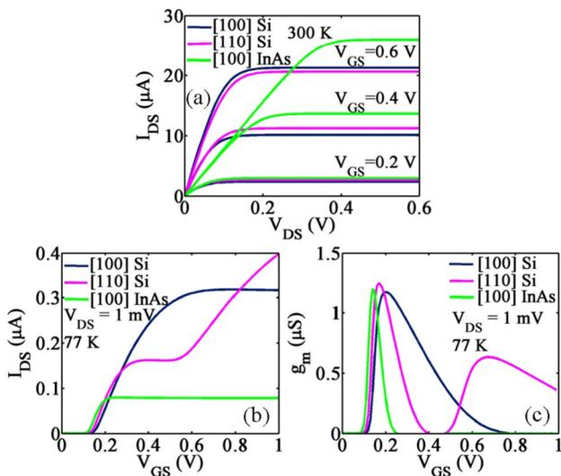
FIG. 5. (a) Simulation results of  $I_{DS}$  vs  $V_{DS}$  of [100] Si, [110] Si, and [100] InAs NWs at  $T=300$  K. The [100] and [110] Si NW results are similar while the InAs NW gives a higher  $I_{on}$  and a lower conductance. Distinctive 1D features are observed in (b)  $I_{DS}$  vs  $V_{GS}$  and (c)  $g_m$  vs  $V_{GS}$  for  $V_{DS}=1$  mV at  $T=77$  K. Two subbands are occupied for the [110] Si NW.
