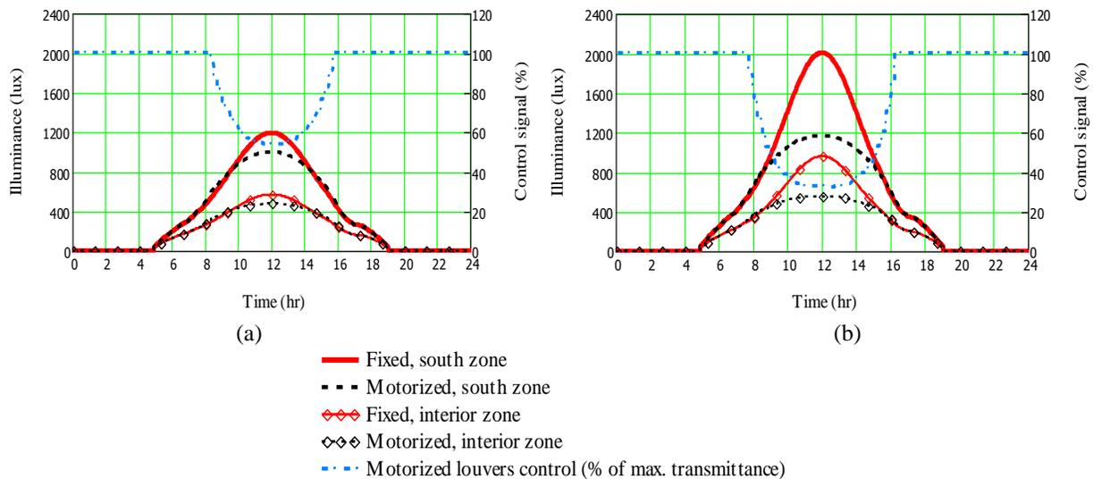
**Figure 8:** Daylight illuminance levels with (a) original daylighting window area (13% WWR) and (b) 40% daylighting WWR, summer
