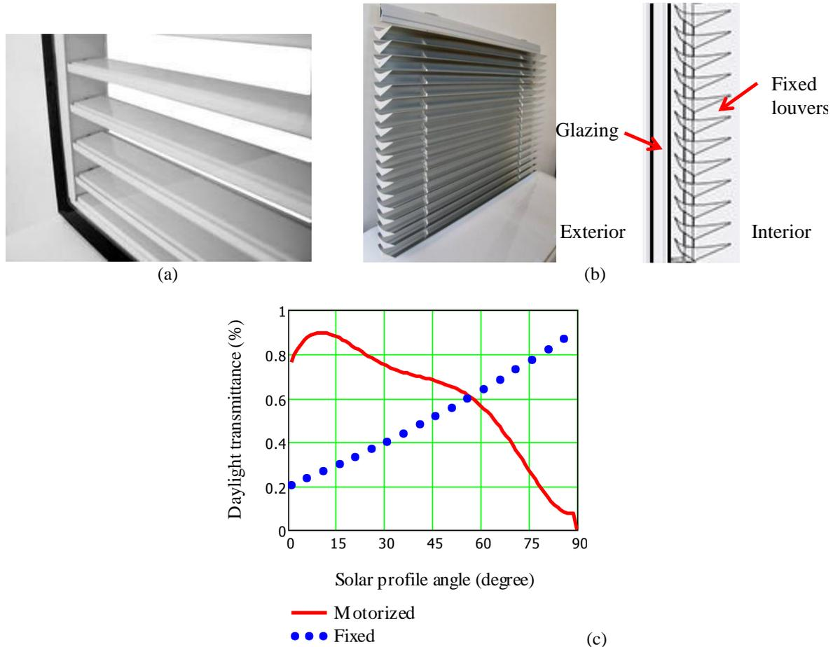
**Figure 1:** Two types of daylight louvers. (a) Motorized daylight louvers between glass panes ([www.unicelarchitectural.com](http://www.unicelarchitectural.com)); (b) Fixed daylight louvers on the interior side of the window ([www.lightlouver.com](http://www.lightlouver.com)); (c) Daylight transmittance (data source for fixed type is [www.lightlouver.com](http://www.lightlouver.com)).
