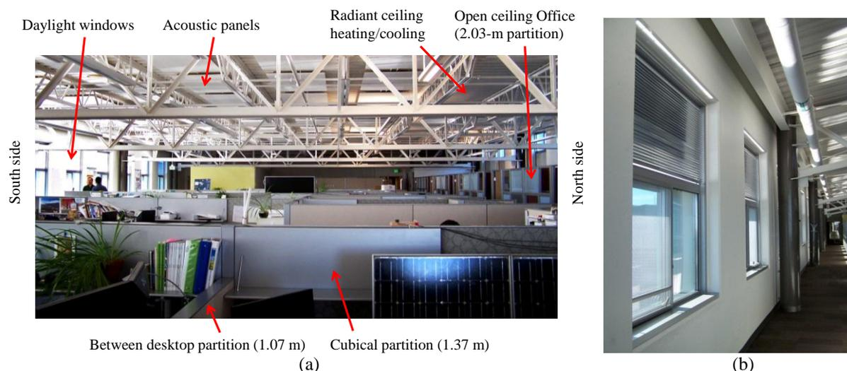
**Figure 2:** (a) Interior space of the typical section, and (b) fixed daylight louvers installed on the interior side of south windows (measured illuminance levels are shown later in Figure 4, for 12:00 P.M.)
