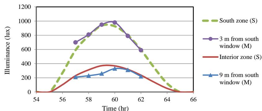
**Figure 4:** Measured (M) and simulated (S) daylight levels on a winter sunny day, Jan 16th, 2013 (3 m is at the common edge of the south zone and the interior zones, 9 m is at the center of the interior zone)
