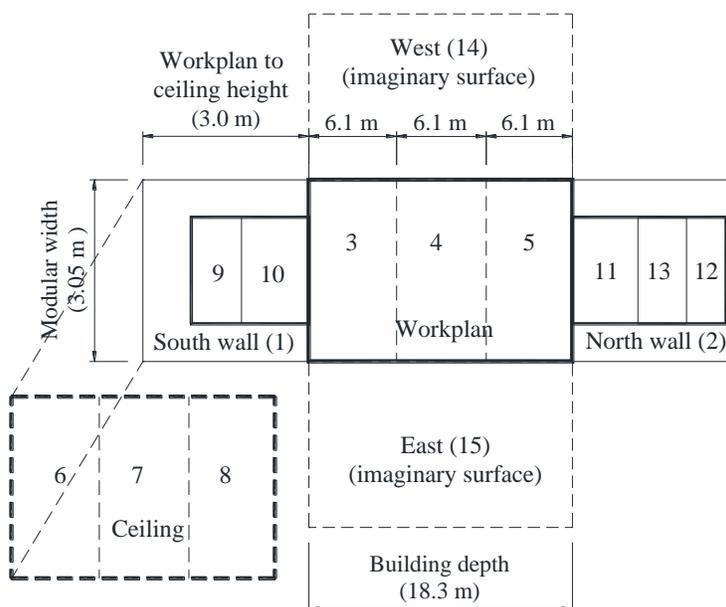
**Figure 3:** Surface division for radiosity calculation.
