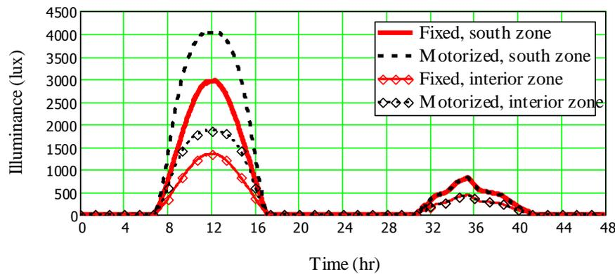
Figure 7: Daylight illuminance levels with 40% daylighting WWR, winter
