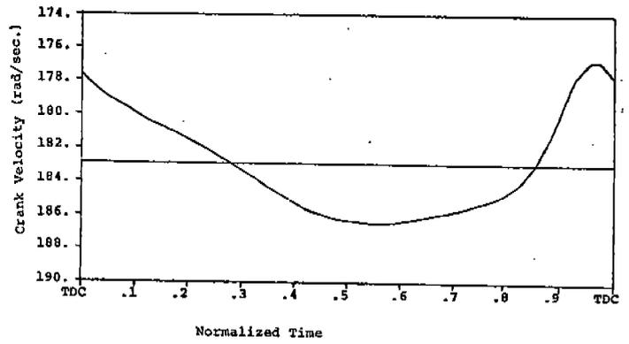
Figure 6. Predicted Steady-State Crank Velocity.
