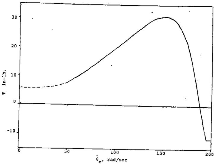
Figure 4. Typical Torque-Speed Curve for 1/4 HP. Shunt-Wound, Single Phase Motor.
