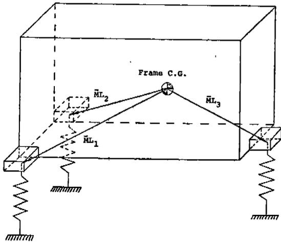
Figure 3. Representation of Positions of Spring Mounting Points and Definition of Mounting Point Locations.
