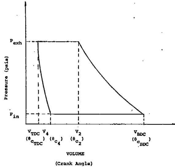
Figure 5. Typical Pressure vs. Volume Curve for Reversible, Polytropic Cycle of an Ideal Gas.
