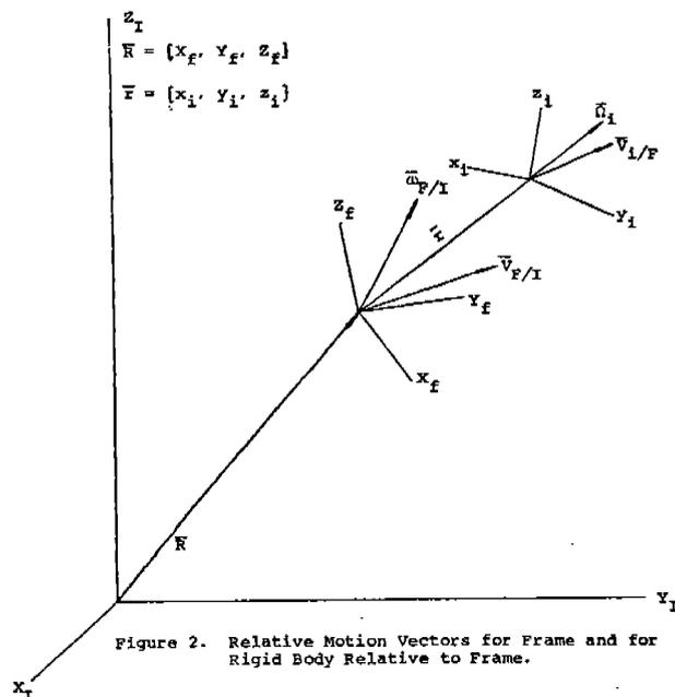
Figure 2. Relative Motion Vectors for Frame and for Rigid Body Relative to Frame.
