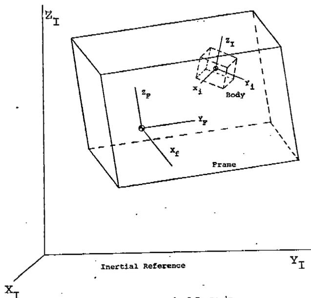
Figure 1. System Composed of Frame in Inertial Reference and Rigid Body Within Frame
