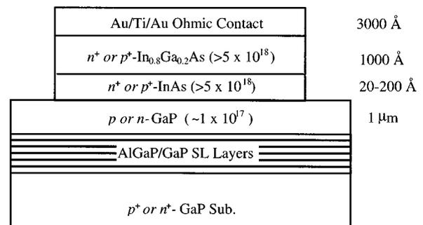
FIG. 1. Illustration of the film structures used for the In<sub>0.8</sub>Ga<sub>0.2</sub>As/InAs/GaP diodes.
