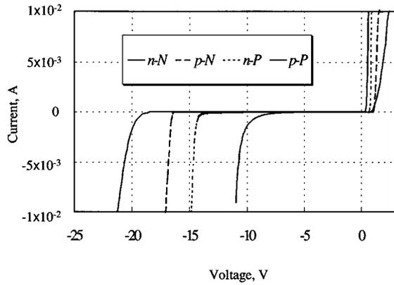
FIG. 2. Linear current vs voltage characteristics of four typical diodes. The size of the diodes was  $90 \times 120 \mu\text{m}^2$  and the measurement temperature was  $23^\circ\text{C}$ .
