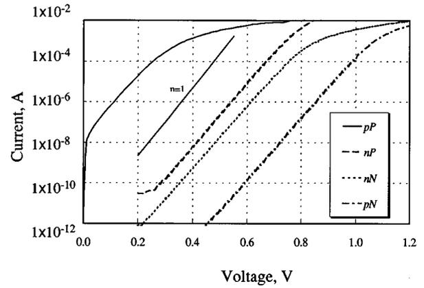
FIG. 3. Logarithmic forward current vs voltage characteristic of the four diodes. The size of the diodes was  $270 \times 360 \mu\text{m}^2$  and the measurement temperature was  $23^\circ\text{C}$ .
