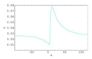
Figure 11. Electron temperature T in eV vs. x in nm at V = 0.28 volts for the medium well RTD: smooth QHD with  $\mu_{n0} = 1000$  cm<sup>2</sup>/(V s) (cyan, light) in the contacts.
