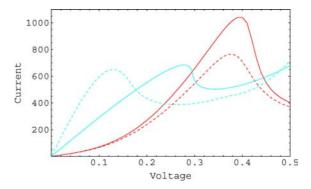
Figure 3. Current in kA/cm<sup>2</sup> vs. applied bias in volts for the thin (3.5 nm) well RTD: NEMO (red, dark), NEMO plus drift-diffusion (dotted red, dotted dark) in the contacts, smooth QHD with  $\mu_{n0} = 1000 \text{ cm}^2/(\text{V s})$  (cyan, light) in the contacts, smooth QHD with  $\mu_{n0} = 2000 \text{ cm}^2/(\text{V s})$  (dotted cyan, dotted light) in the contacts.
