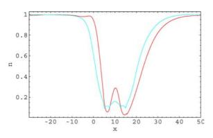
Figure 6. Electron density n in  $10^{18}$  cm<sup>-3</sup> vs. x in nm at V = 0.15 volts.
