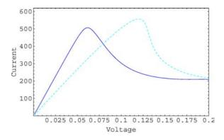
Figure 4. Current in kA/cm² vs. applied bias in volts for the medium well RTD: smooth QHD with constant  $\tau_p = \tau_w$  (blue, dark) in the contacts, corresponding to a constant mobility  $\mu_n = 2000 \text{ cm}^2/(\text{V s})$ , compared with smooth QHD with  $\mu_{n0} = 2000 \text{ cm}^2/(\text{V s})$  (dotted cyan, dotted light) in the contacts.
