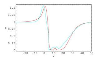
Figure 10. Electron density n in  $10^{18}$  cm<sup>-3</sup> vs. x in nm at V = 0.35 volts.
