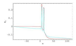
Figure 5. Conduction band energy  $E_c$  in eV vs. x in nm at V=0.15 volts for the medium well RTD: for Figs. 5–10 NEMO (red, dark) with 30 nm contacts, smooth QHD with  $\mu_{n0}=1000$  cm<sup>2</sup>/(V s) (cyan, light) in the 100 nm long contacts.
