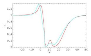
Figure 8. Electron density n in  $10^{18}$  cm<sup>-3</sup> vs. x in nm at V = 0.28 volts.
