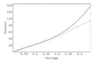
Figure 1. Current in kA/cm<sup>2</sup> vs. applied bias in volts for the single 5 nm barrier diode: NEMO (red, dark), smooth QHD with  $\mu_{n0} = 1000 \text{ cm}^2/\text{(V s)}$  (cyan, light) in the contacts.
