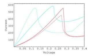
Figure 2. Current in kA/cm<sup>2</sup> vs. applied bias in volts for the medium (5 nm) well RTD: NEMO (red, dark), NEMO plus drift-diffusion (dotted red, dotted dark) in the contacts, smooth QHD with  $\mu_{n0} = 1000 \text{ cm}^2/(\text{V s})$  (cyan, light) in the contacts, smooth QHD with  $\mu_{n0} = 2000 \text{ cm}^2/(\text{V s})$  (dotted cyan, dotted light) in the contacts.
