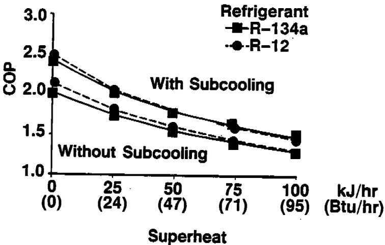
Figure 4. Comparison of COP values for R-134a and R-12 at equal cooling duty (-21°C/+43°C)
