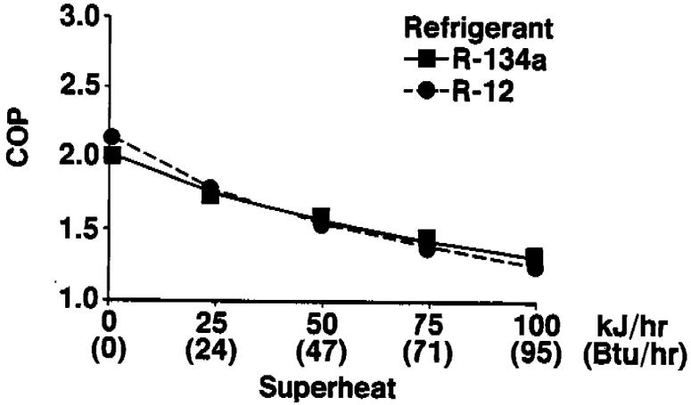
Figure 3. Comparison of COP values for R-134a and R-12 at equal cooling duty (-23°C/ +54°C)
