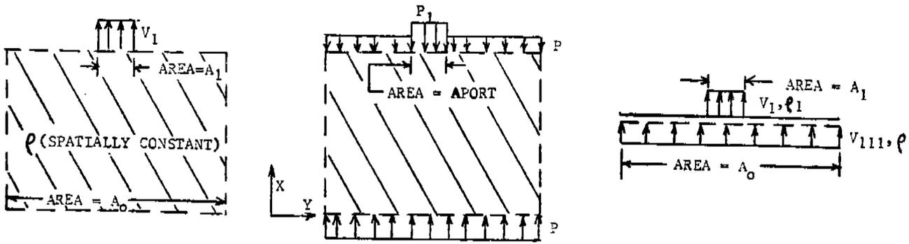
FIG. 2a ASSUMED VELOCITY AND PRESSURE PROFILES FOR CONTROL VOLUME  $V_0$
