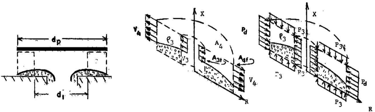
FIG. 2d VELOCITY AND PRESSURE PROFILES, CONTROL VOLUME  $V_3$
