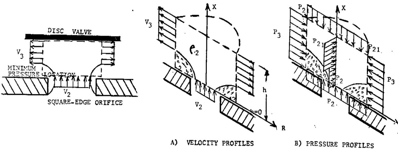
FIG. 2c ASSUMED VELOCITY AND PRESSURE PROFILES, CONTROL VOLUME  $V_2$
