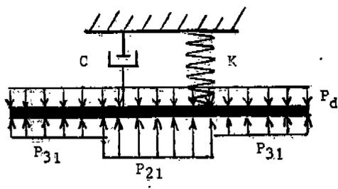
FIG. 3 MECHANICAL SPRING DISC VALVE SYSTEM
