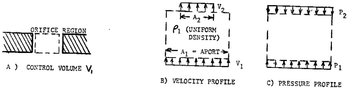
FIG. 2b VELOCITY AND PRESSURE PROFILES ACROSS THE SQUARE-EDGE ORIFICE BOUNDARY
