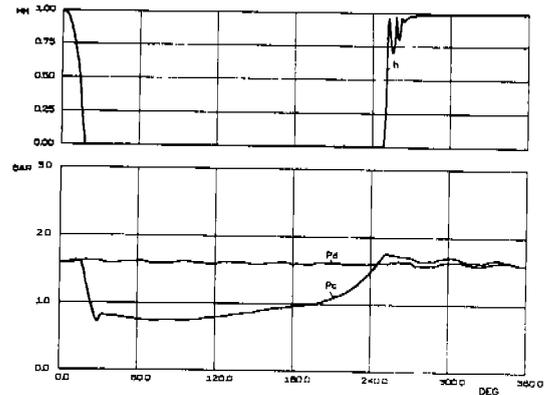
Fig. 7 Typical experimental result. Discharge valve operated without springs. Compressor speed 400 rpm.
