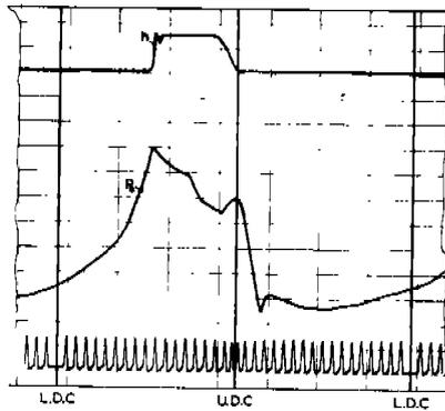
Fig. 13 Experiment recording of discharge test valve fitted with springs calculated by eqs. 4 and 5.  $C_s = 6000$  N/m. Compressor speed 850 rpm.
