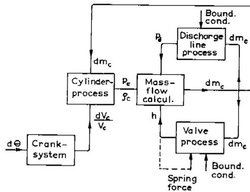
Fig. 8 Schematic block-diagram of discharge valve process
