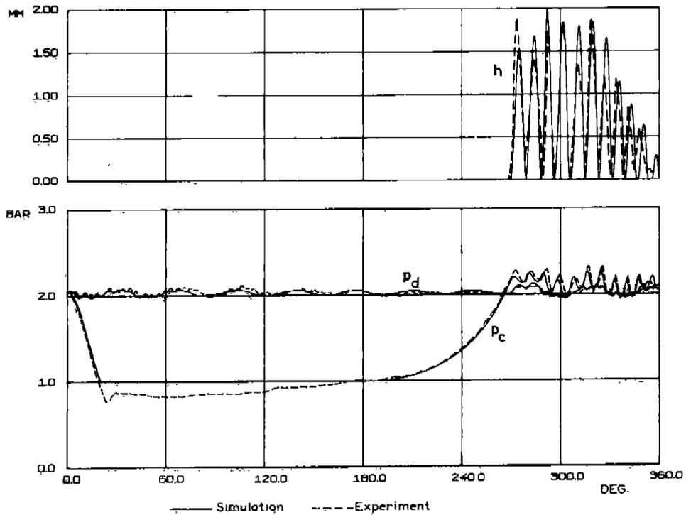
Fig. 9 Comparison of experiments and computer simulation for discharge valve operated with springs. Compressor speed 400 rpm.
