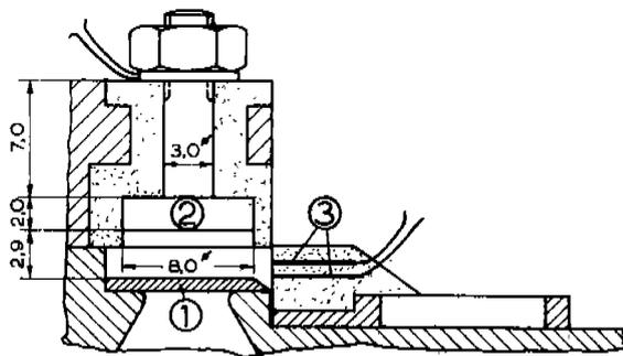
Fig. 2 Displacement transducer arrangement
