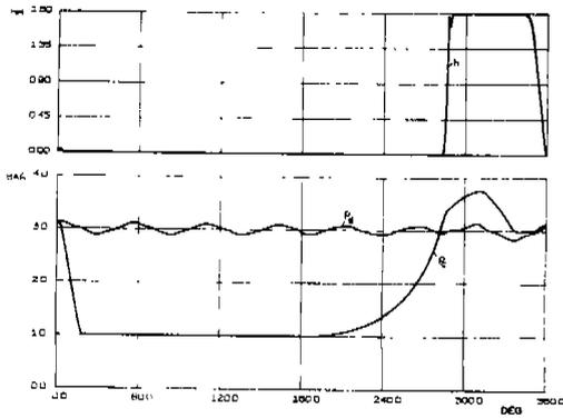
Fig. 11 Computer simulation of a discharge valve process. Valve springs designed according to eqs. 4 and 5. Compressor speed 600 rpm.
