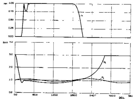
Fig. 12 Computer simulation of a suction valve process. Valve springs designed according to eqs. 4 and 5. Compressor speed 1450 rpm.
