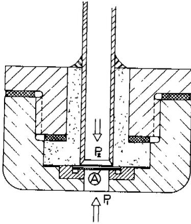
Fig. 4 Pressure calibration pick-up
