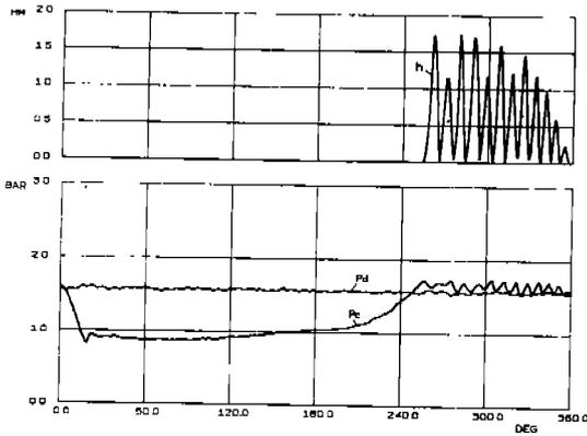
Fig. 6 Typical experimental result. Discharge valve operated with springs ( $F_{SO}=12 \text{ N}$ ,  $C_S=11400 \text{ N/m}$ ). Compressor speed 400 rpm.
