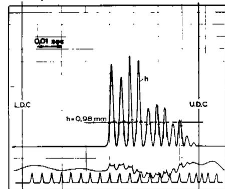
Fig. 3 Calibration of valve lift signal
