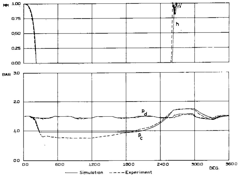
Fig. 10 Comparison of experiments and computer simulation for discharge valve operated without springs. Compressor speed 800 rpm.
