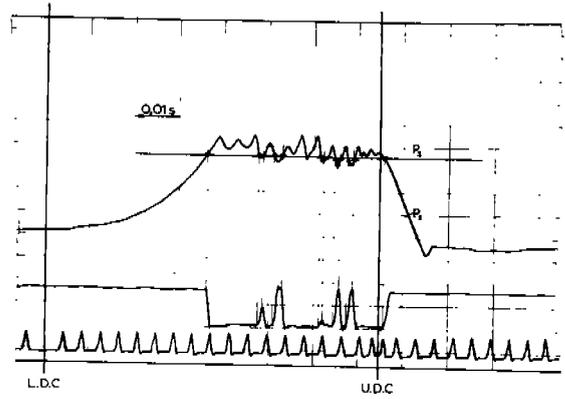
Fig. 5 Calibration of signal from the cylinder pressure transducer
