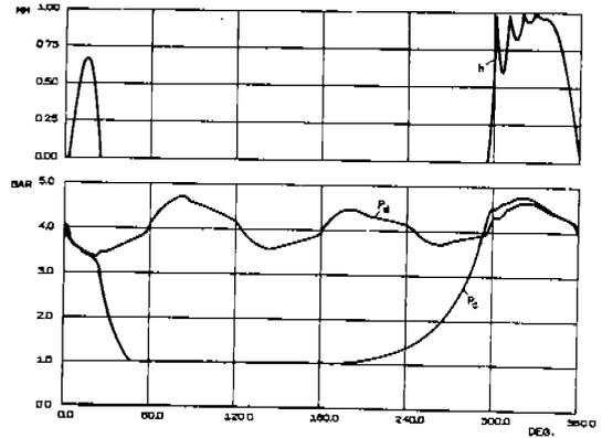
Fig. 14 Computer simulation demonstrating possible influence of discharge line pressure oscillations on the valve behaviour. Discharge line length 1.38 m. Comp. sp. 1450 rpm.
