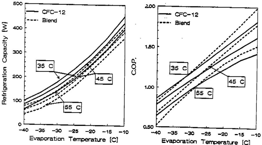
Figure 1. Comparison of the COP and the refrigeration capacity: Comparison of the COP and the refrigeration capacity of the three component blend and CFC-12 versus evaporation temperature (superheat, subcooling and ambient temperature equal to 32 C)
