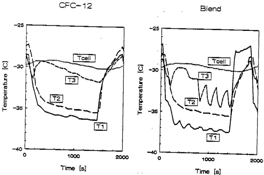
Figure 3. Time dependent registration of evaporator temperatures during an on/off cycle: Various temperatures on the evaporator (upper, middle and lower position referred to as 1, 2 and 3) and the average air temperature (referred to as the cell temperature) are given for measurements using either the three component blend or CFC-12.
