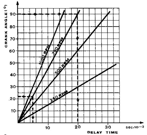
FIG. 2 - CORRESPONDENCE BETWEEN CRANK ANGLE, TIME AT VARIOUS RPM
