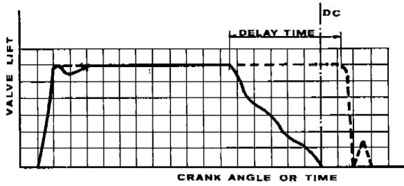
FIG. 1 - COMPARISON OF ANALYTICAL DISPLACEMENTS WITH (---) AND WITHOUT (—) OIL STICKING EFFECT
