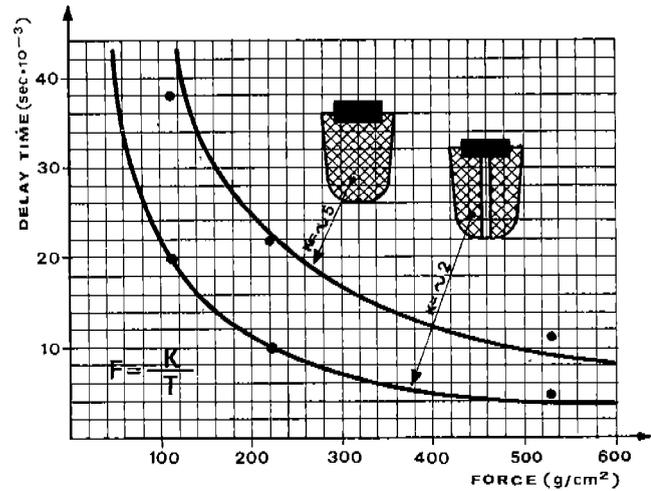
FIG. 6 - DELAY TIME-SPECIFIC FORCE CORRELATION OF DIFFERENT VALVE STOPS FOR ABUNDANT LUBRICATION
