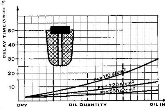
FIG. 5a - DELAY TIME CORRELATION WITH SPECIFIC FORCES AND OIL QUANTITY FOR VALVE STOP WITH HOLES
