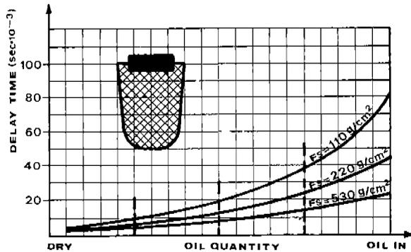
FIG. 5b - DELAY TIME CORRELATION WITH SPECIFIC FORCES AND OIL QUANTITY FOR VALVE STOP WITHOUT HOLES
