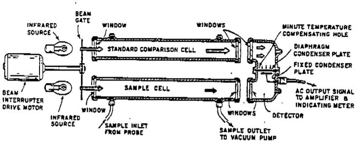
Figure 2. Infrared Leak Detector
