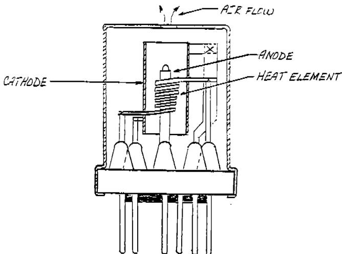
Figure 1. Gas Ionization Detector Cell
