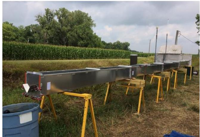
**Figure 2.** 10-m flume used in the constant injection study.
