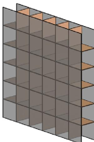
**Fig.2.** Double glazed window with grid shading component
