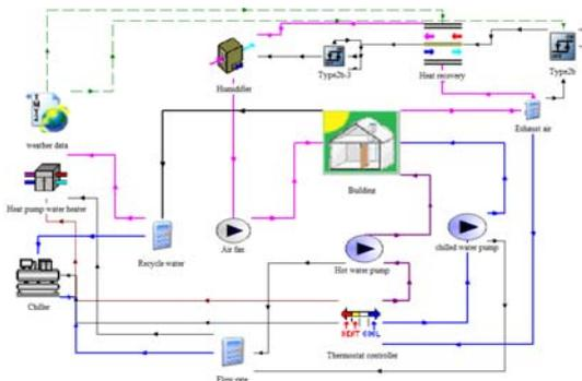
**Fig.4.** Case2 prototype model without CFS components
