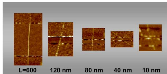
FIG. 1 (color online). Atomic force microscopy (AFM) images of five devices consisting of individual SWNTs with lengths in the range of  $L = 600$  to  $10$  nm between the edges of Pd contact electrodes.
