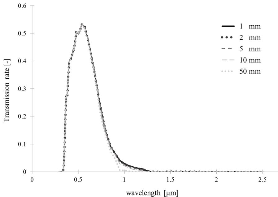
**Figure 6:** Transmission rate vs. wavelength, for different thicknesses of the fluid layer
