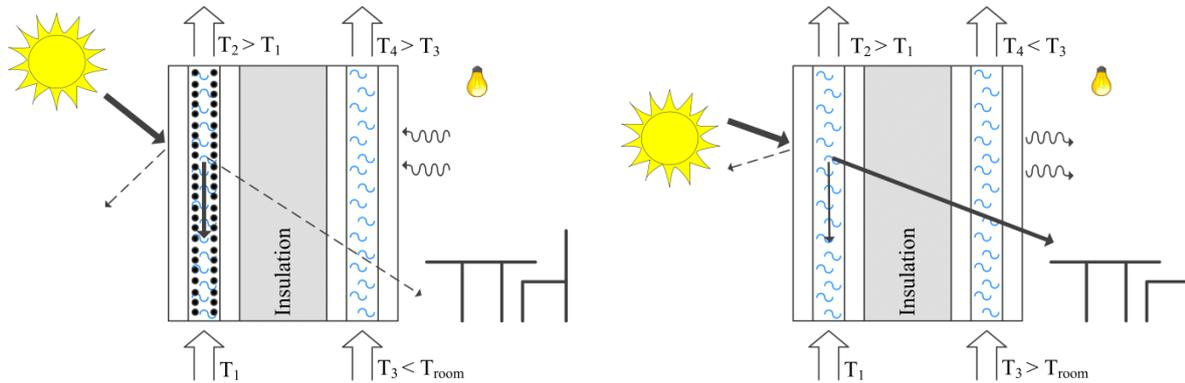
**Figure 2:** Basic operating modes of the fluidglass in summer (left) and winter (right)
