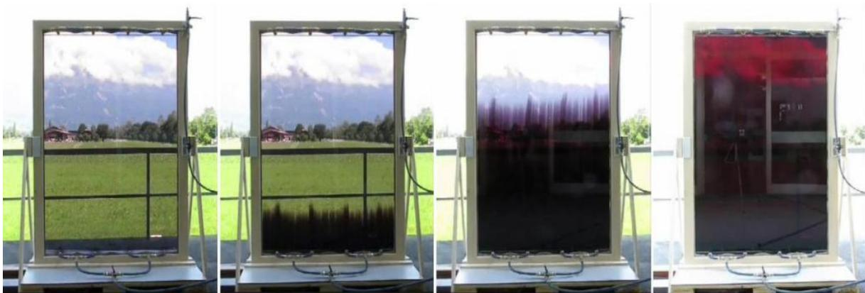
**Figure 8:** Preliminary tests using a colorant to vary the absorptivity, for total shading
