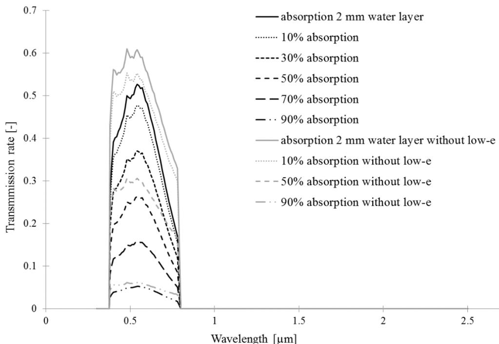
Figure 7: Ideal fluid with different absorption rates
