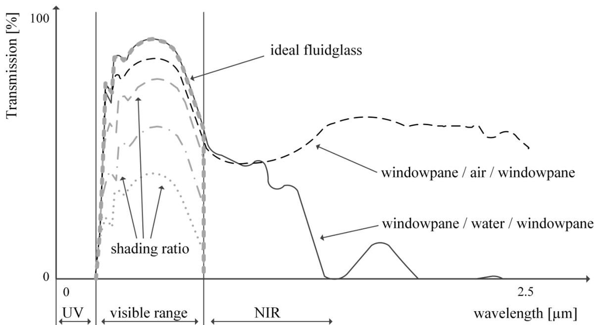
**Figure 3:** Transmission rate of windowpanes, filled with air, filled with water and for the ideal fluidglass with several shading values.
