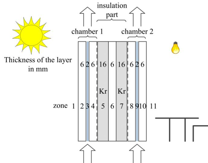
**Figure 4:** Glazing system consisting of two fluid chambers separated by an insulation glass unit in the middle
