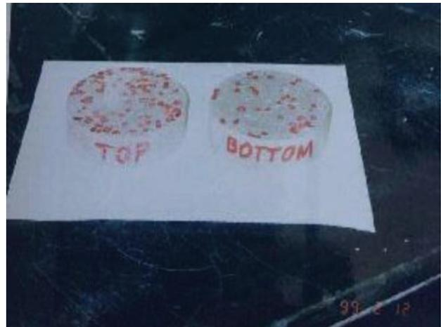
Figure 16. Marked surface aggregate with size larger than 5 mm.
