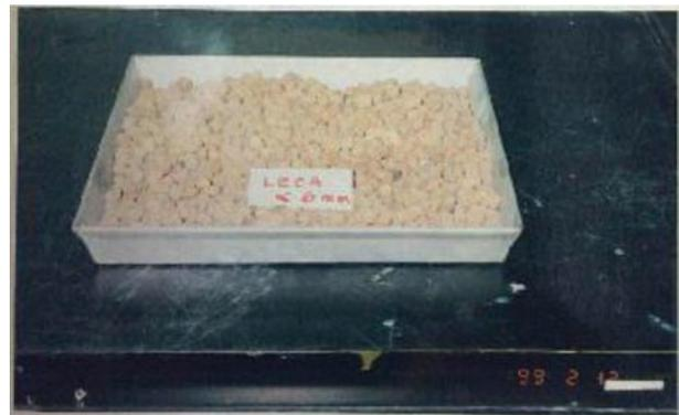
Figure 1. Lightweight aggregate-leca with size <6 mm.
