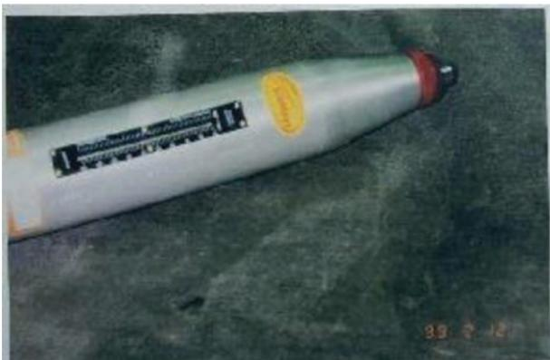
Figure 12. Rebound Hammer-Type L.
