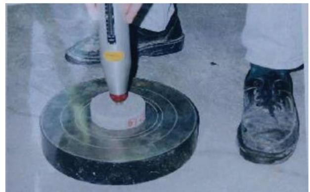
Figure 17. A setup of Rebound Hammer test.
