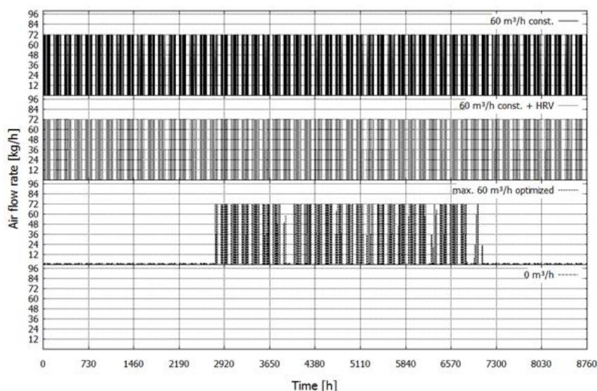
**Figure 4:** Annual hourly air flow rate of mechanical ventilation for the WSchV 82 building
