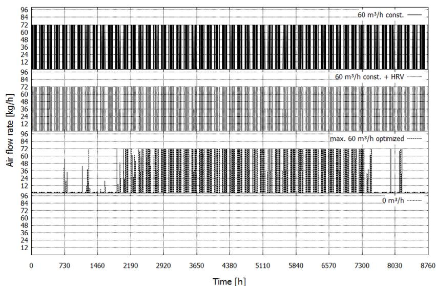
**Figure 3:** Annual hourly air flow rate of mechanical ventilation for the EnEV 2009 building
