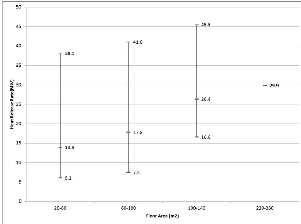
**Figure 2:** Minimum, average and maximum heat release rates for flashover to occur in different-sized flats
