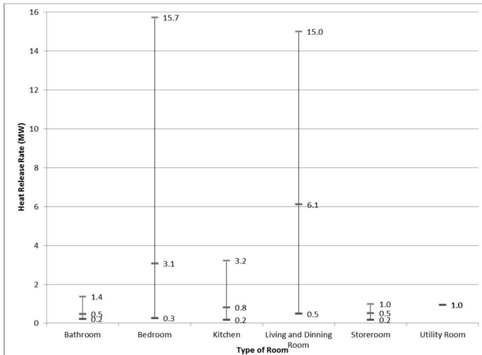
**Figure 3:** Minimum, average and maximum heat release rates for flashover to occur in different types of rooms
