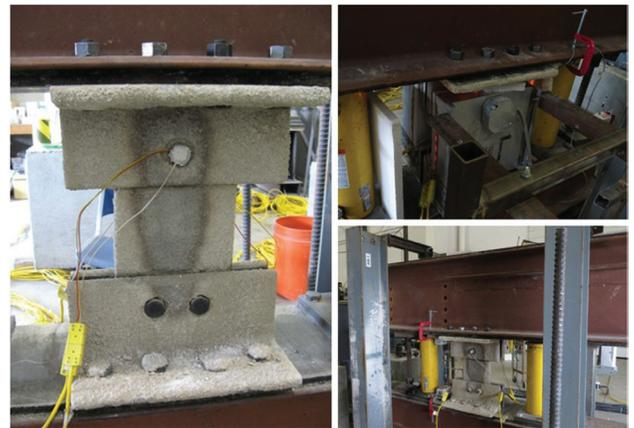
Throughout the project, the test specimen (left) was used for full-scale experimental tests as well as the heaters (top right), together forming the full test setup (bottom right).
