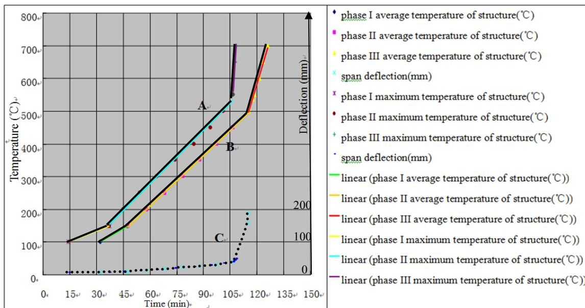
Figure 8: Temperature-time-deflection curve of verification test on thick coating
