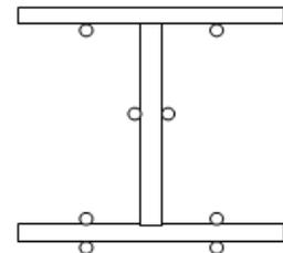
**Figure 1:** Structural members in the tests**Figure 2:** Measurement positions of H-type section thickness
