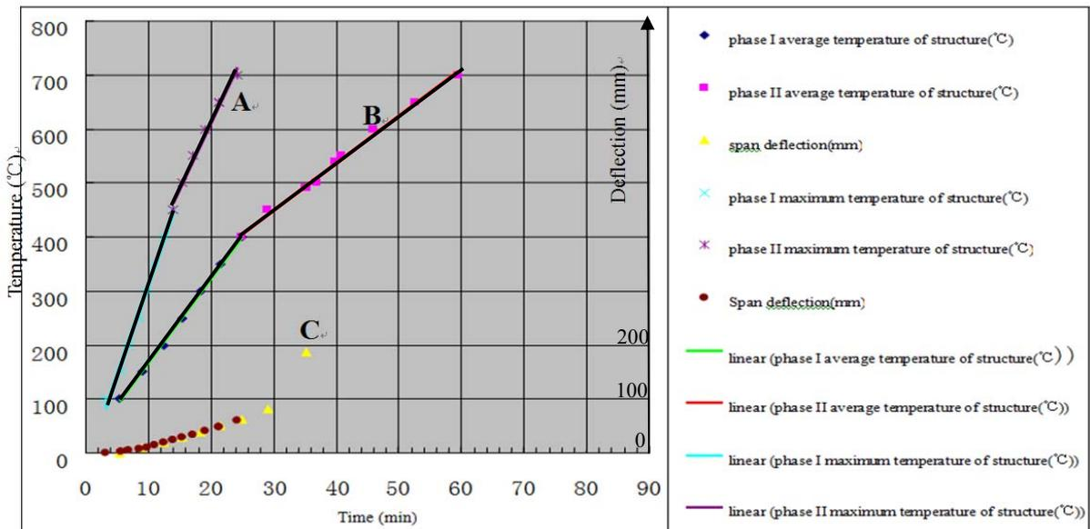
Figure 6: Temperature-time-deflection curve of main test on thin coating
