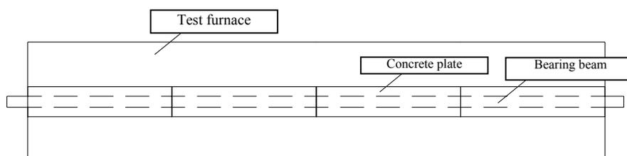
**Figure 3:** Layout of bearing beam test part inside the furnace
