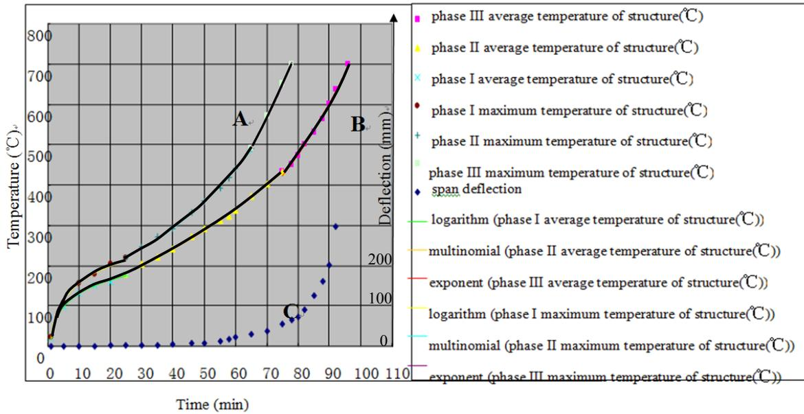
Figure 5: Temperature-time-deflection curve of verification test on ultra-thin coating
