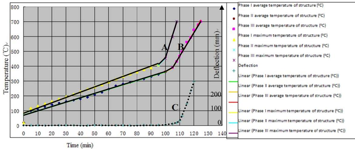
Figure 7: Temperature-time-deflection curve of verification test on thin coating
