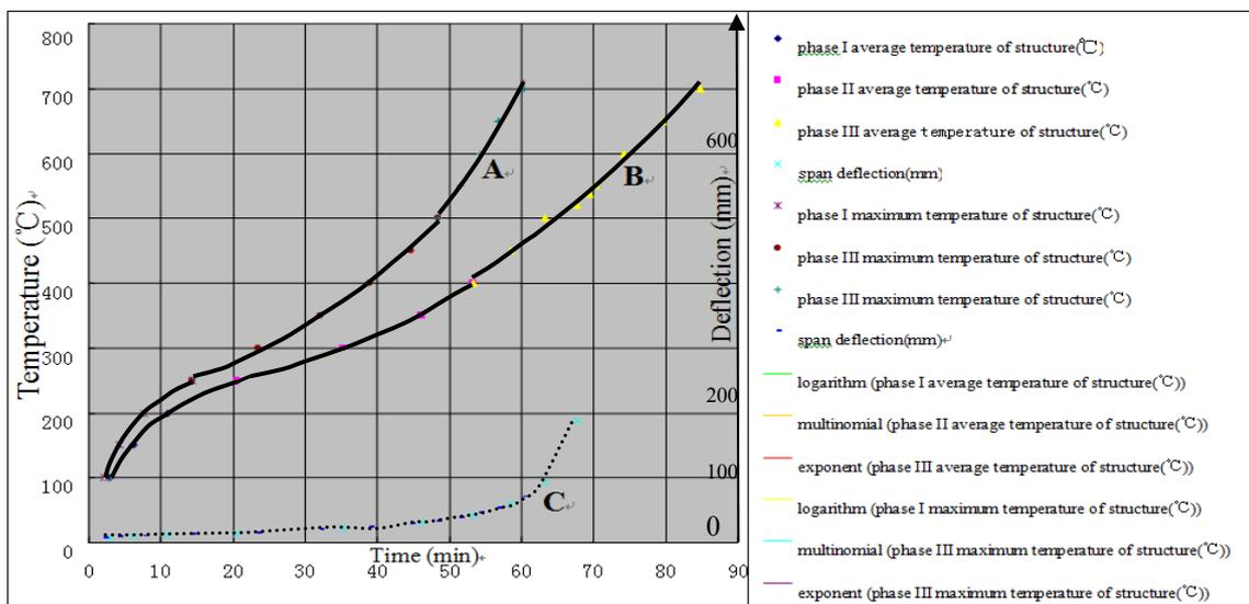
Figure 4: Temperature-time-deflection curve of main test on ultra-thin coating
