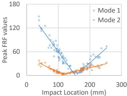
Figure 1a. The peak FRF as a function of impact location for Bat 2. (The distal end of the bat is 0 mm.)
