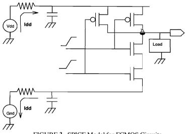
FIGURE 3. SPICE Model for FCMOS Circuits
