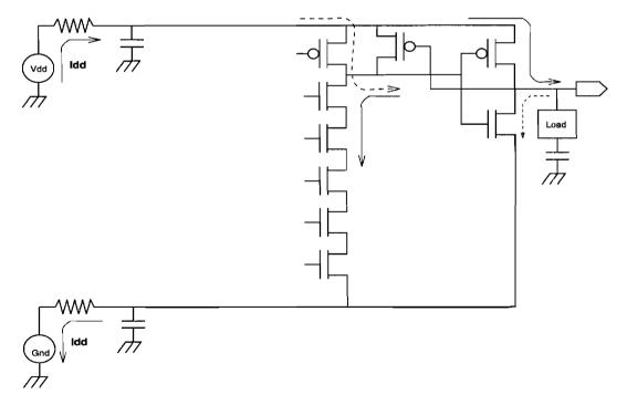
FIGURE 10. Simulation setup to obtain  $I_{\mbox{\scriptsize DD}}$  waveforms for domino logic
