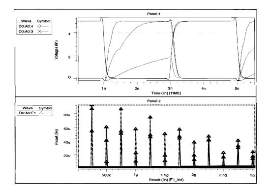
FIGURE 5. Simulations for a resistive short at the drain of the PMOS of an inverter gate
