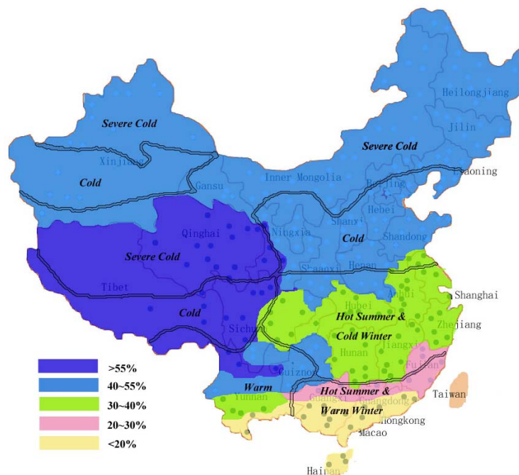
Figure 4: The energy-saving distribution map of the thermosyphon heat exchanger in China
