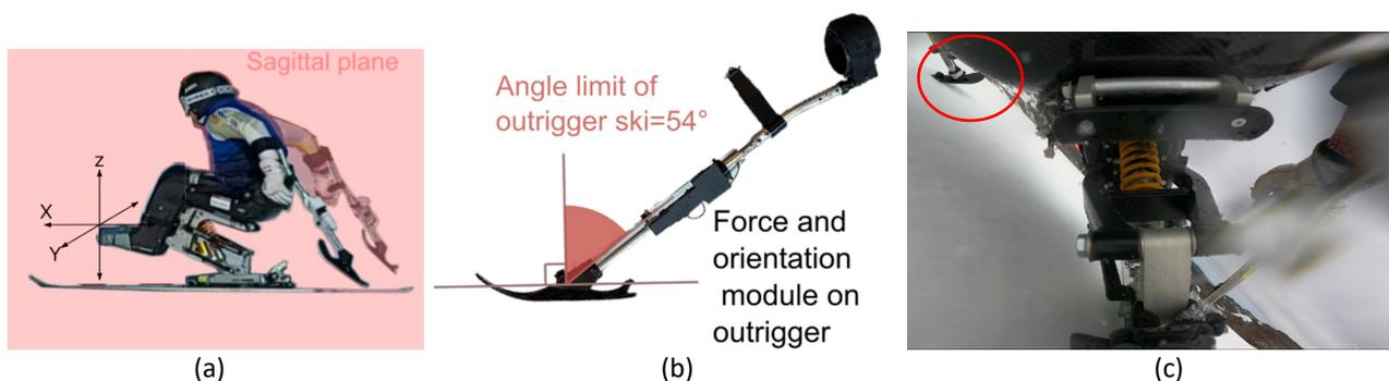
Fig. 1: a) Sagittal plane of the sit-ski and the coordinate system. b) Flip-type sensor outrigger-ski with the 54° rotation limitation. c) Outrigger-ski 90° relative to the sit-ski while collecting data, above 54° limitation.
