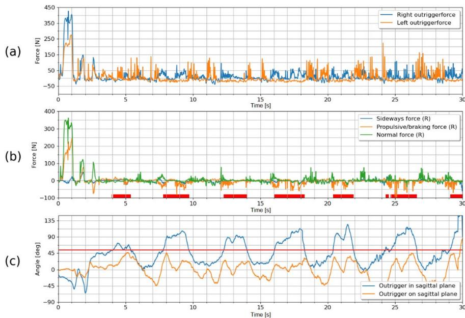
Fig. 2: a) Axial-force measurements from right and left outrigger. b) Decomposed forces of the right outrigger-ski relative to the sit-ski. Red rectangles shows where the outrigger angle is over the angle limit of the outrigger-ski. c) Orientation of the right outrigger-ski relative to the sagittal plane of the sit-ski with a red line at 54°.
