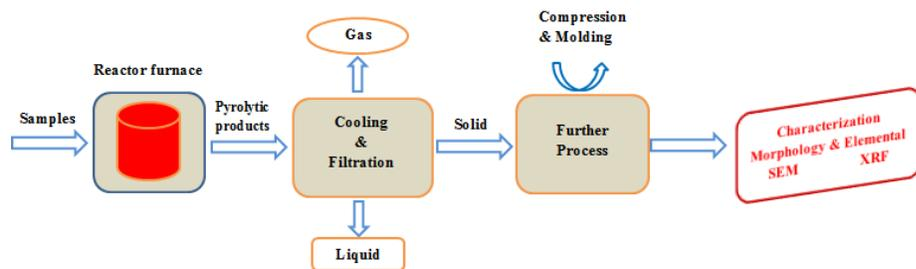
**Figure 2.** The pyrolysis process setup.
