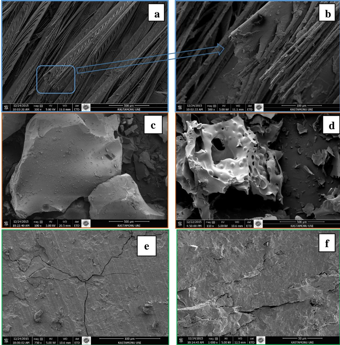
**Figure 3.** SEM images of a & b - unprocessed chicken feathers at two magnifications, c & d - pyrolysis of solid powder at two different temperatures (400 & 650° C), and e & f - surface and fractured surface of compressed chicken feather material (650° C).
